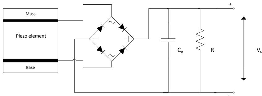
**Figure 15: A “typical” energy harvesting circuit, same as above but with an added resistor that represents the system resistance**
