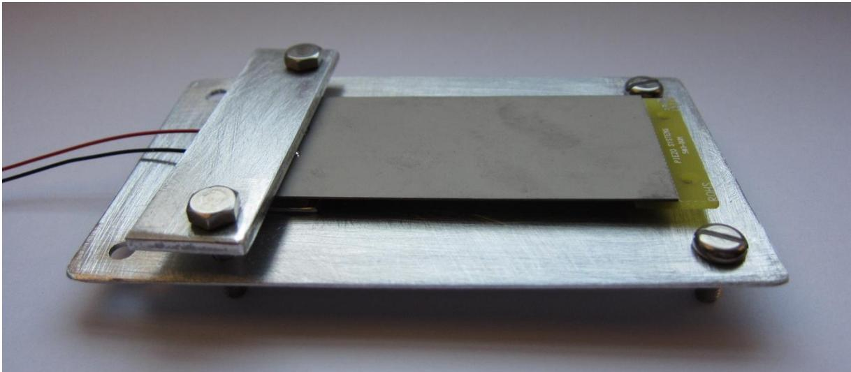
**Figure 28: The PZT plate with a mount that enables testing by fastening points and also protects the plate from too large tip deflections**
