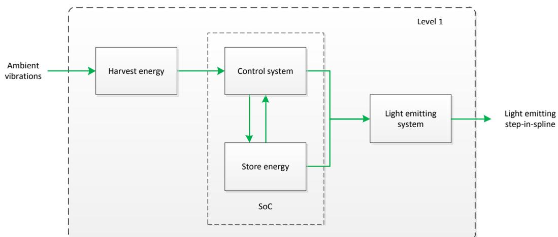
Figure 12: First level of the functional model for a piezoelectric solution
