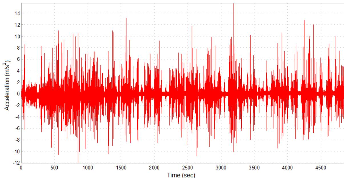
**Figure 10: Vertical acceleration data – city driving 35km, car model: S80, year model 2000.**
