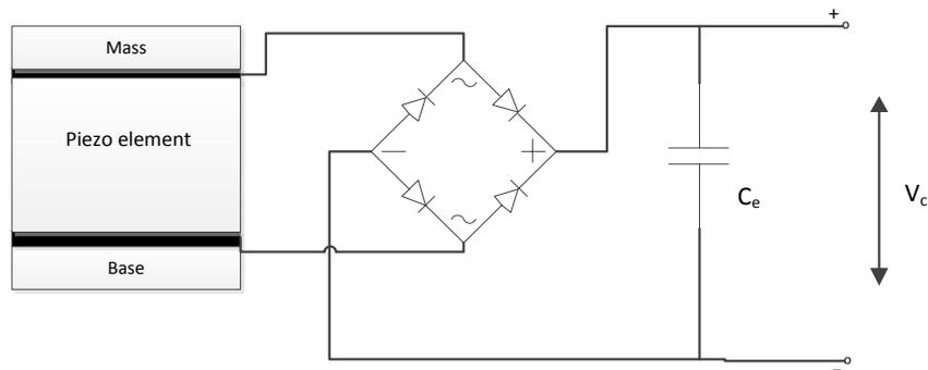
Figure 14: The energy harvester circuit to begin the tests with
