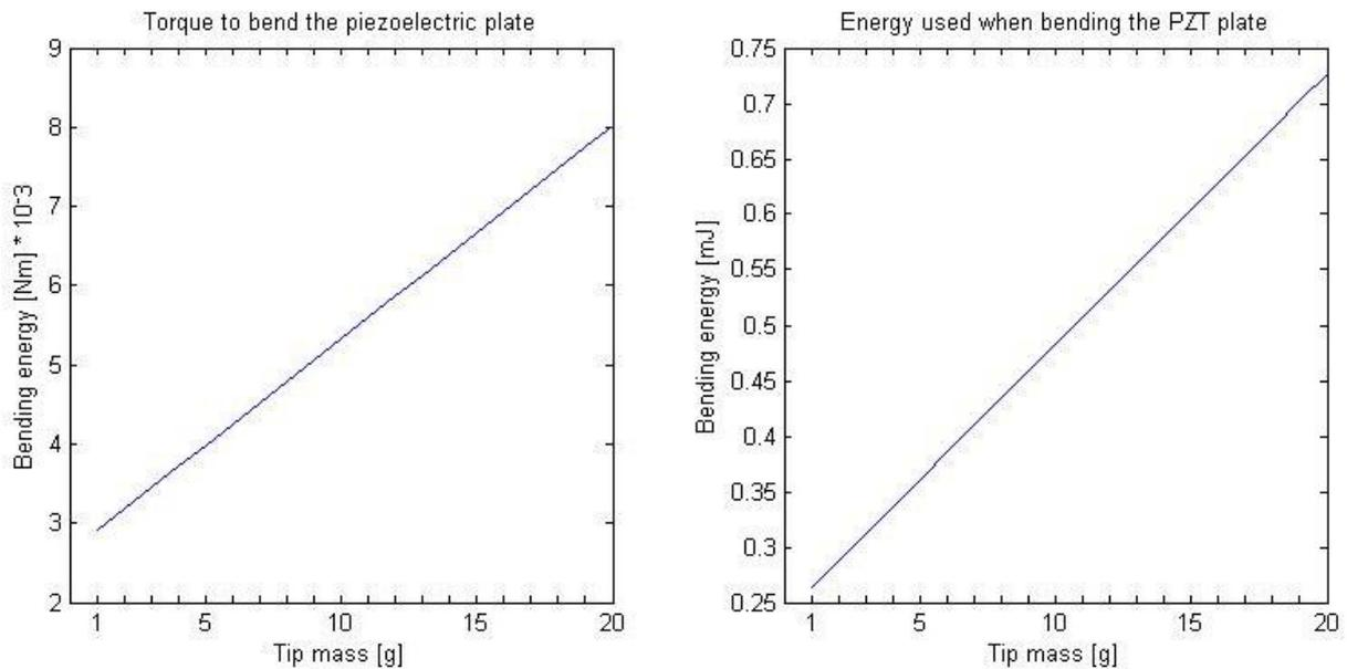
**Figure 27: Beam bending energy with varying tip mass**
