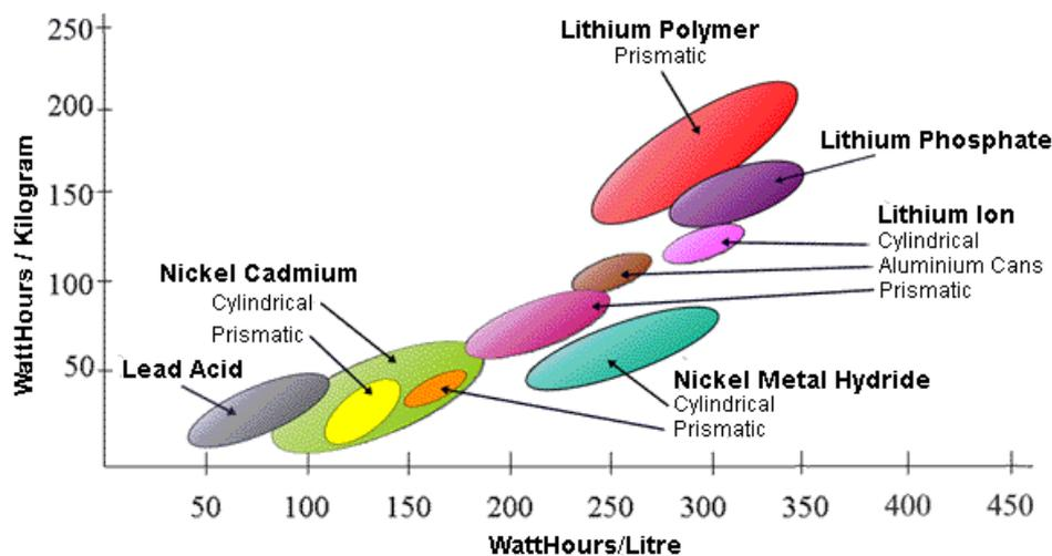
Figure 20: Relative energy density of some common secondary cell chemistries (from Woodbank Communications Ltd.)
