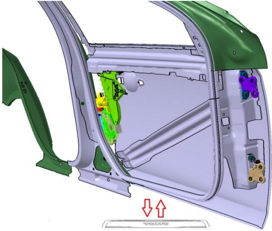
Figure 39: The relative force from the door that “bounces” on the piezo element
