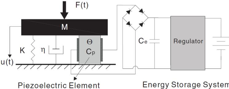
Figure 40: The piezoelectric energy harvesting model used in calculations by Shu & Lien (2006)
