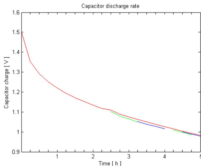
**Figure 30: Discharge rate of the capacitors after the logical circuit malfunctioned (a plot with larger time frame can be found in the appendix)**
