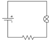
**Figure 33: The circuitry used to get a relationship between charge and illumination time**
