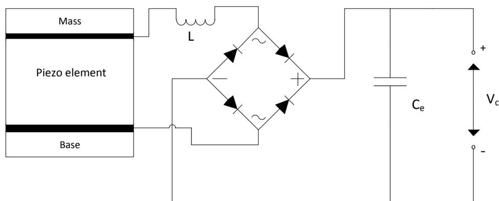
**Figure 16: The "typical" energy harvester with an inductor implemented in the circuitry**
