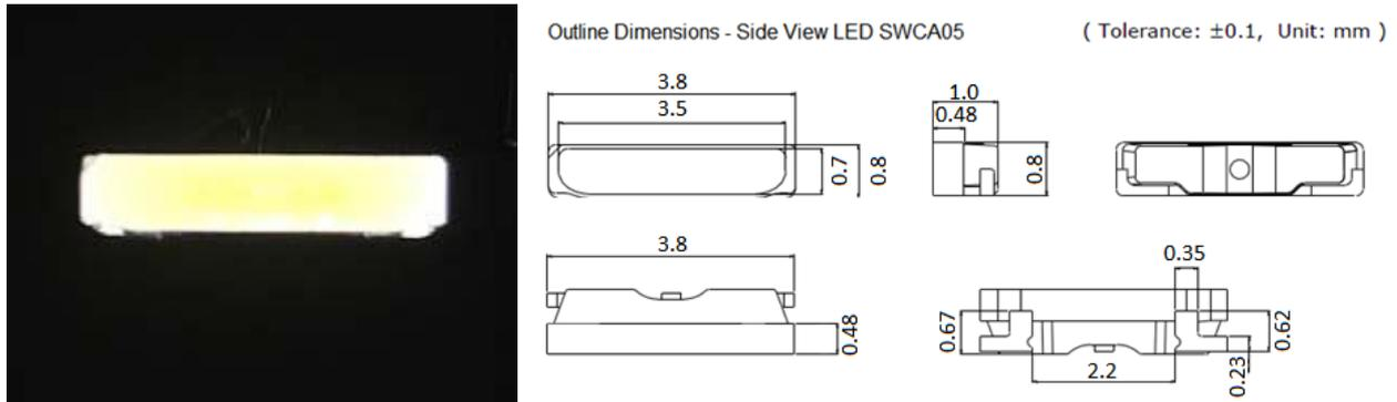
Figure 19: The side view LED used within the step-in-spline today
