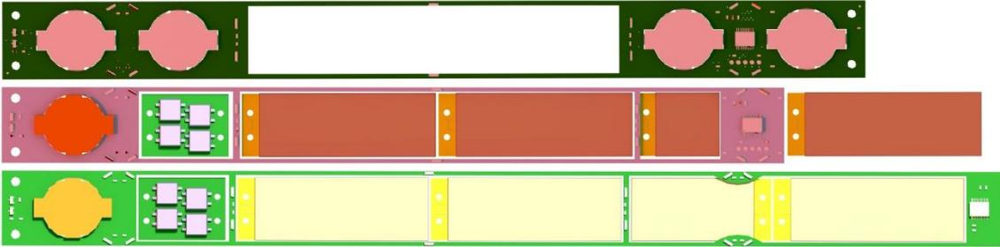
Figure 22: Electric circuitry of today (top) compared to a slightly modified piezoelectric solution (middle) and a longer circuitry proposition that can contain four big piezo-plates (bottom).
