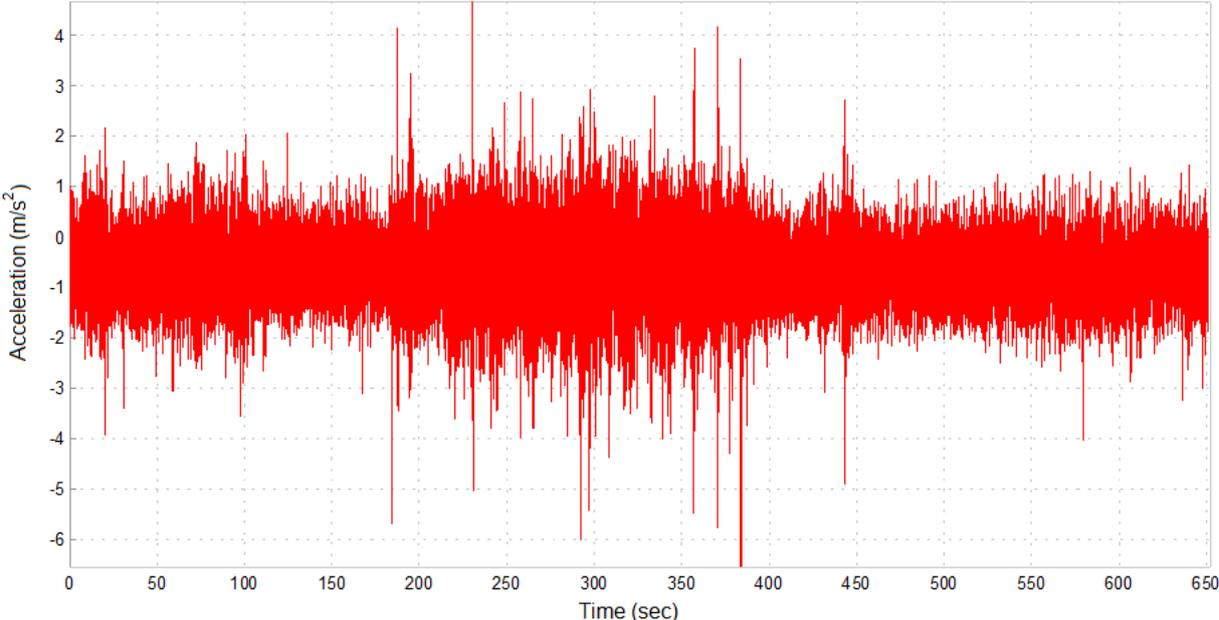
Figure 36: Vertical acceleration data – motorway 22km, car model: S80, year model 2000.
