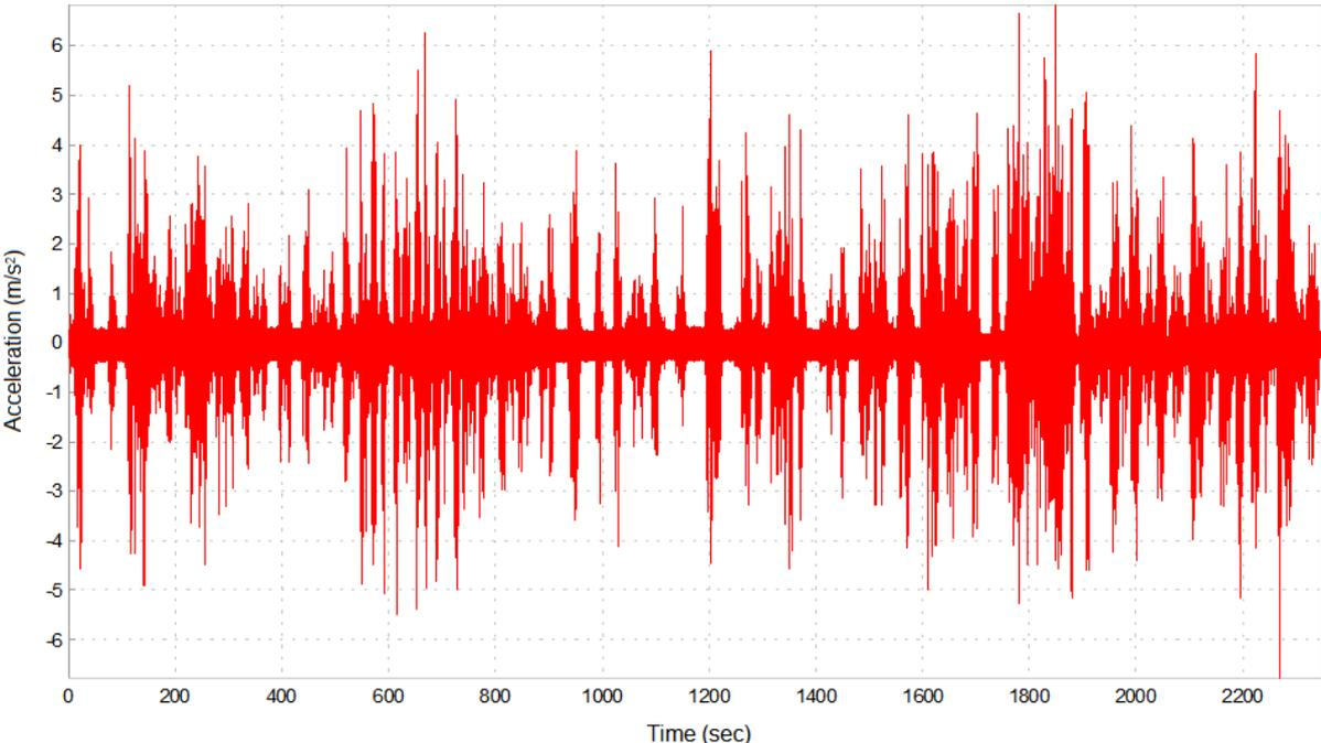
Figure 37: Vertical acceleration data – regular driving, car model: S80, year model 2000.
