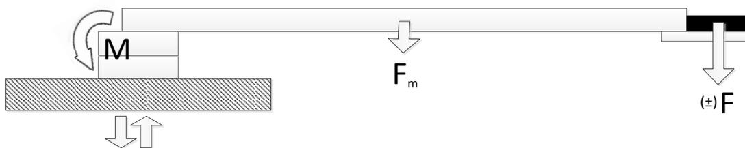
Figure 26: The cantilever mount of the piezoelectric material 5A4E with its affecting forces illustrated
