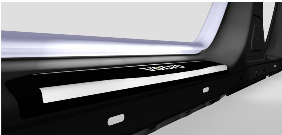
**Figure 5: The illuminated step-in-spline as part of the interior styling**
