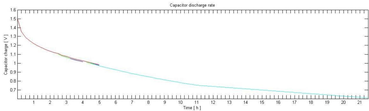
The figure shows the discharge rate during a period of 21½ hours
