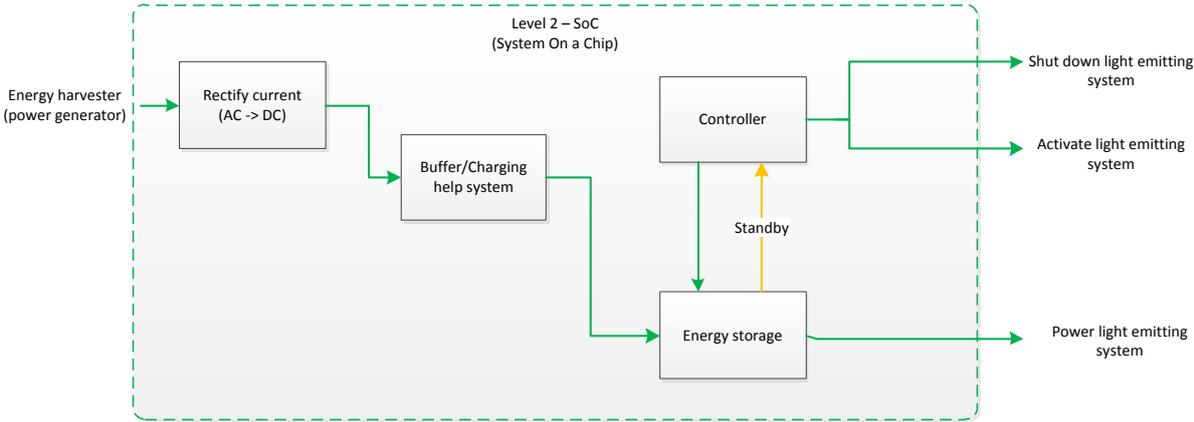
**Figure 13: Level 2 of the functional model, where the circuitry is in focus**
