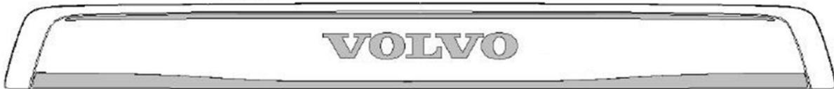
Figure 6: The step-in-spline with lights, the dark areas are illuminated.
