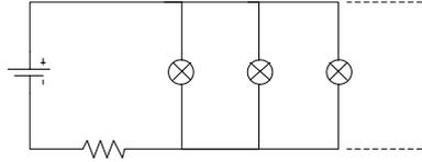
**Figure 34: The theoretical circuitry used when approximating the charging time with more than one diode**
