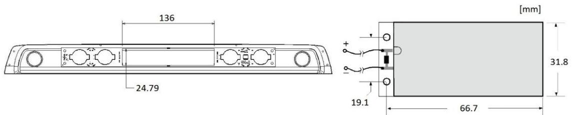
**Figure 21: The available space for piezo plates within the unmodified step-in-spline (left), and 503-standard piezo-plate dimensions from Piezo Systems Inc. (right)**
