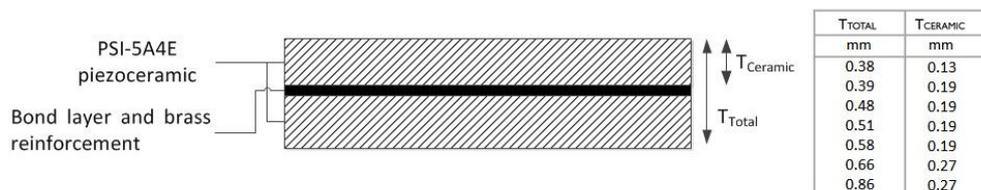
Figure 25: Height information of the piezo material chosen for the prototype
