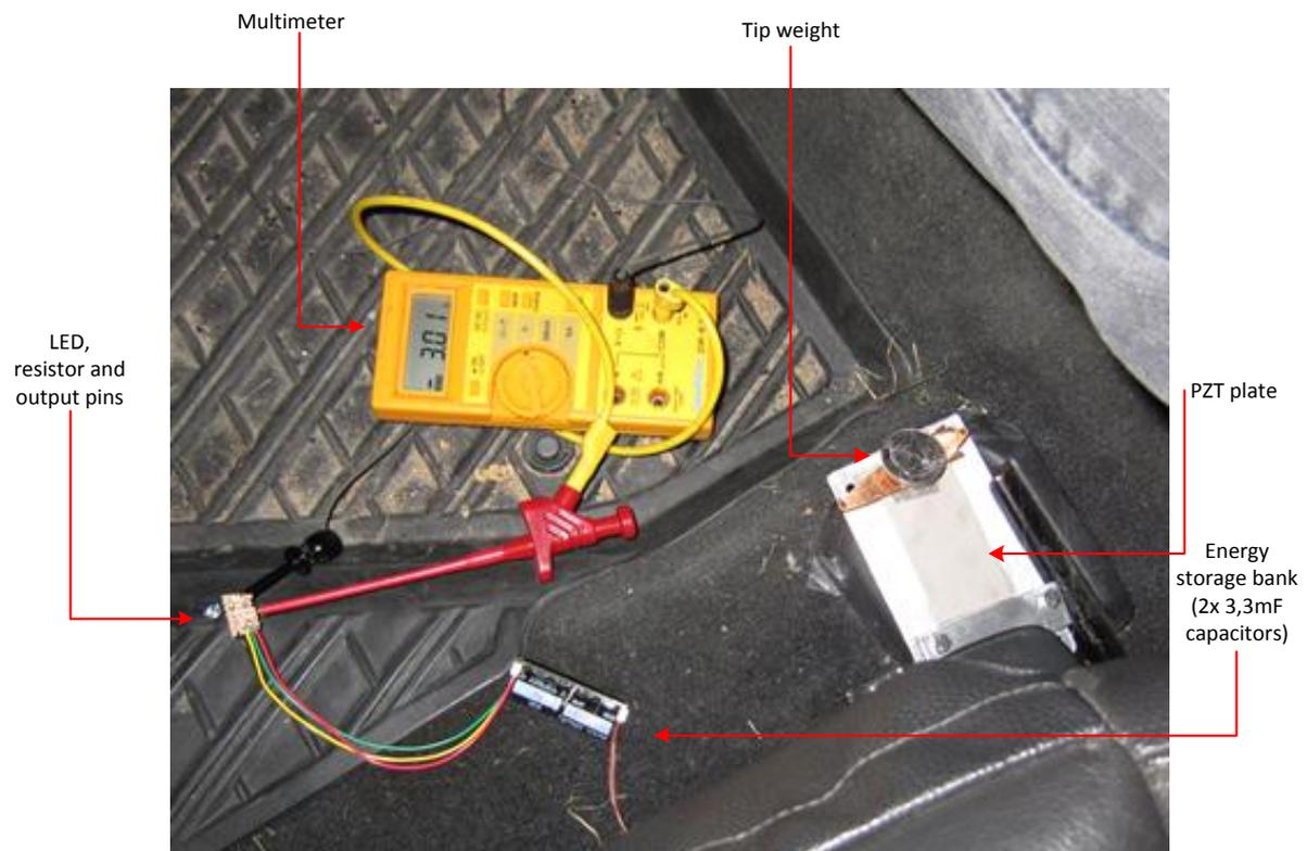
Figure 29: Initial test system
