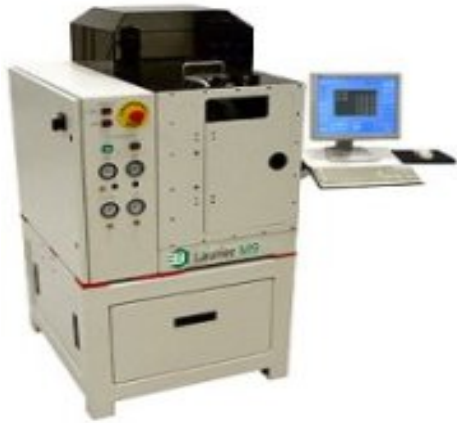
Fig. 26. Flip chip bonding machines performing thermocompression for gold-to-gold bonding. (a) The bonder at NCTU. (b) The bonder at Chalmers.
