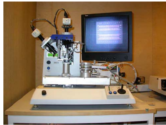
Fig. 26. Flip chip bonding machines performing thermocompression for gold-to-gold bonding. (a) The bonder at NCTU. (b) The bonder at Chalmers.
