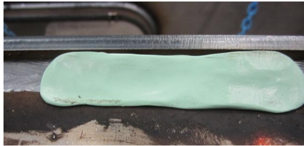
Figure 9: Polymer applied to weld to get impressions.
