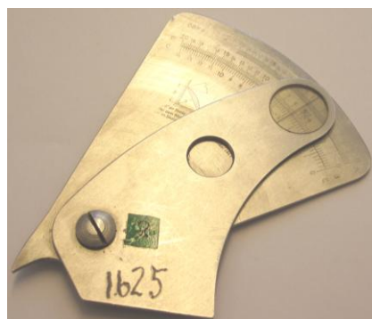
Figure 3: Throat size gauge used at the plant.
