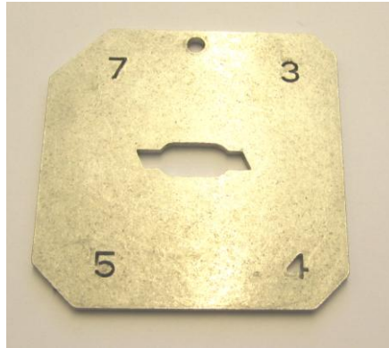
Figure 5: Gauge measuring throat size using corner chamfering.
