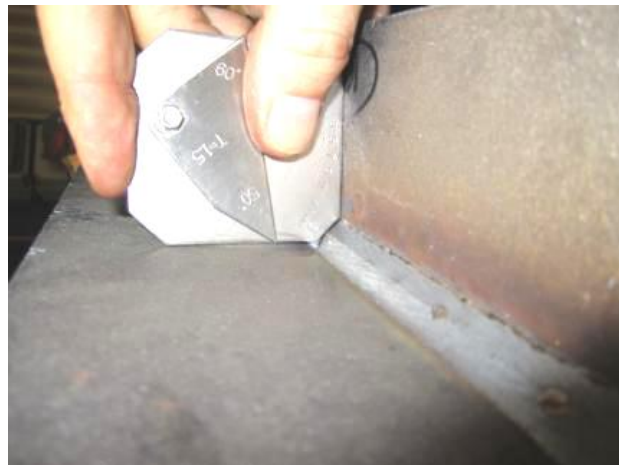
Figure 4: Tool for deciding weld shape.
