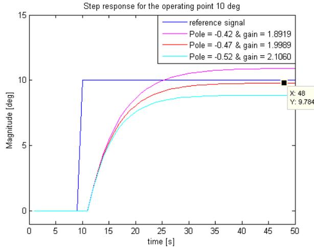
Figure 5: Shows the step response of the system with different pole placements
