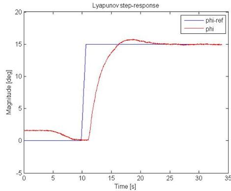
Figure 16: Validation using Lyapunov control
