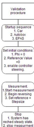
Figure 15: Start sequence of the experiment
