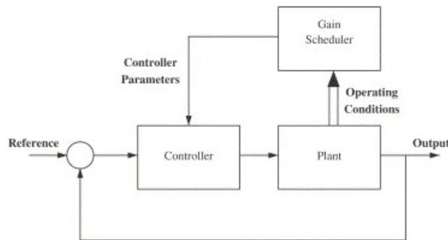
Figure 4: A schematic of the closed-loop system using a gain scheduling controller
