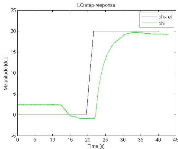
Figure 17: Validation using LQ control
