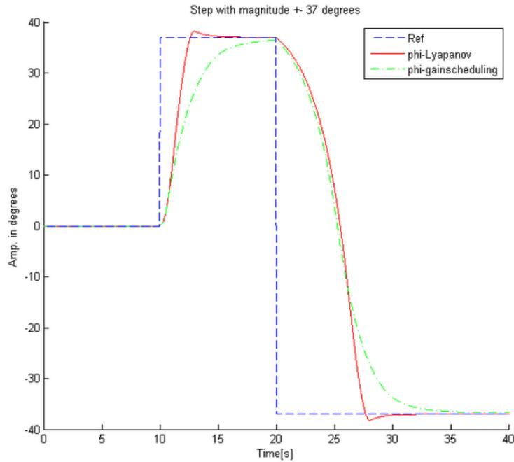
Figure 9: Comparison between Lyapunov control and gain scheduling control
