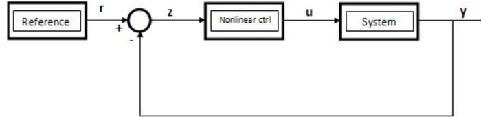
Figure 6: A schematic of the closed-loop system using Lyapunov controller
