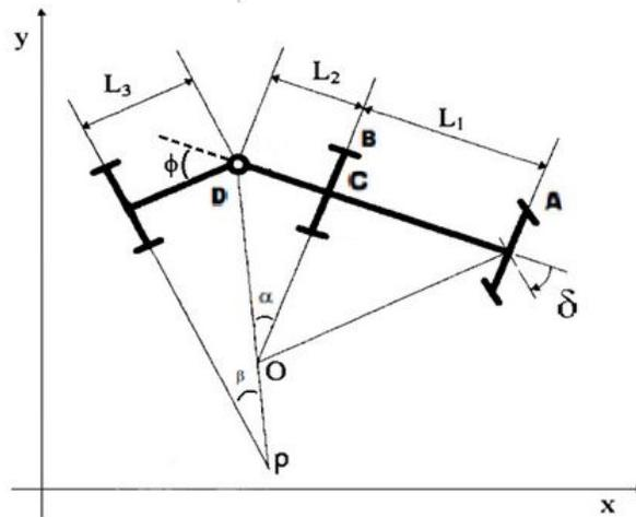
Figure 2: Model of the articulated vehicle
