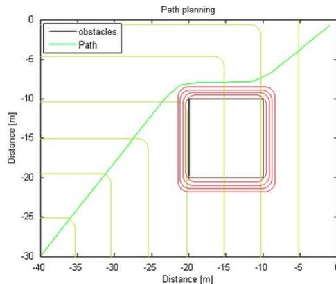
Figure 11: Trajectory given as input to the system. Green level curves indicate attractive forces and red indicates repulsive forces.
