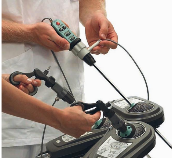
Figure 1.3 Simball4D , which is the system Surgical Science is currently using. The position of the instrument is determined by encoding a pattern on the ball which the instrument is attached to.
