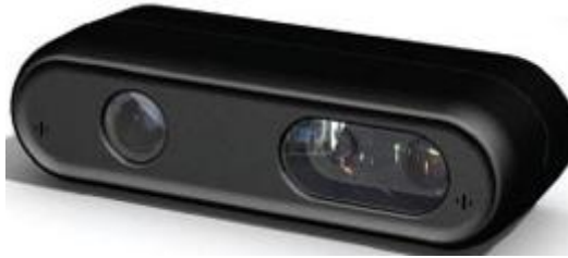
Figure 3.16 PrimeSensor is a camera system which is used e.g. in game control unit Xbox kinect controller.
