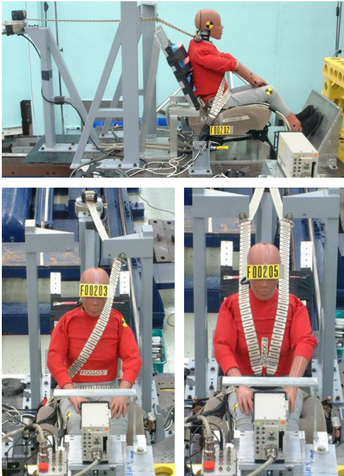
Figure J-8 Rouhana test setup with a Hybrid III 5F dummy. Top and bottom left; 3pt belt system, bottom right 4-pt belt (photos from the preparation of the tests used in the reproduction of the tests by Rouhana et al. 2003)
