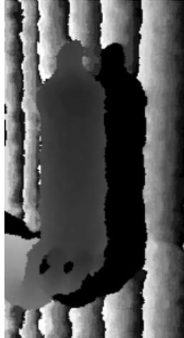
Figure 1.3.3: A bottle captured using a Kinect camera to illustrate the loss of information in the shadow cast by the object being captured.
