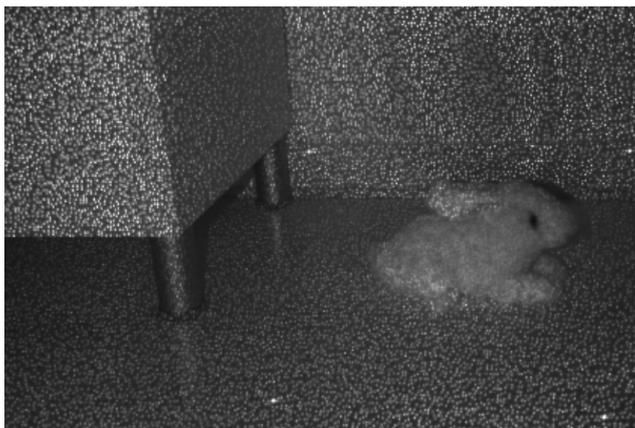
Figure 1.3.2: *IR image of the projected light pattern produced by a Kinect Sensor.*
