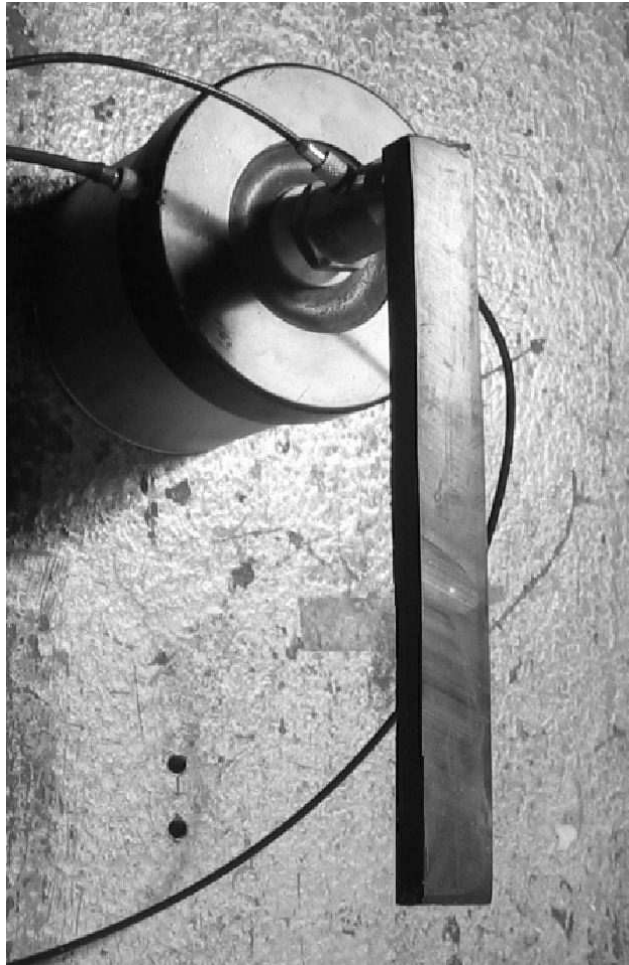
Figure 4.18: Figure depicts the measurement setup which had the rubber sample placed directly on an impedance head.
