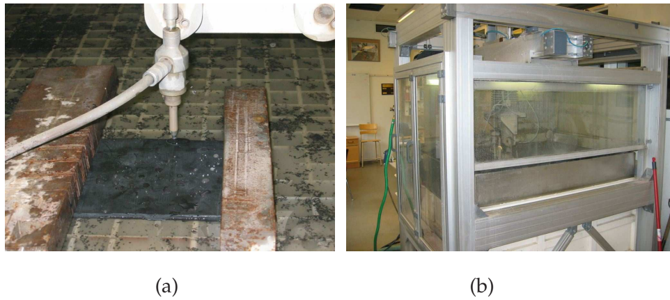
Figure 4.8: (a) shows the water jet cutter in the progress of cutting a sample. (b) shows the encapsulation from the outside.
