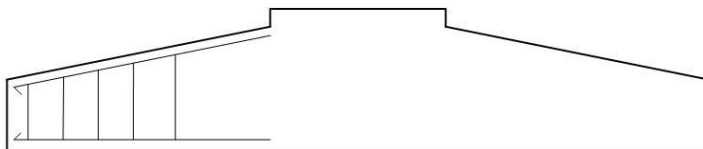
Figure 2.2. Bending reinforcement is placed in the top and in the bottom of the structure and shear reinforcement is placed as vertical stirrups.
