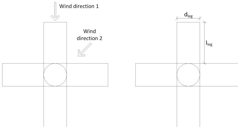
Figure 2: Four-legged stocky structure. Calculations are performed for two different wind directions
