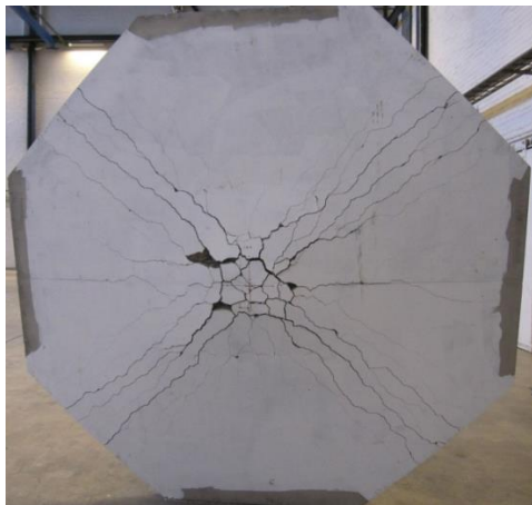
Figure 4.10 Crack pattern from experiment
