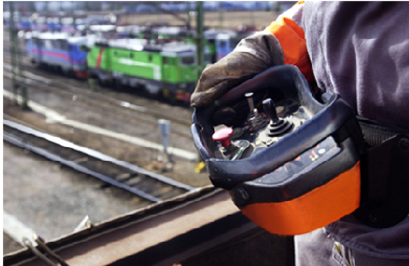
Figure 28: A shunter using a control transmitter to remotely control an engine. (Åkerströms, 2013)
