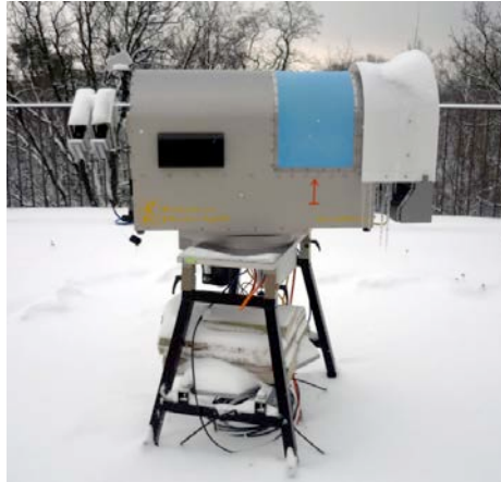
Fig. 2. RPG-HATPRO MWR capable to estimate both air temperature and water vapor vertical profile.
