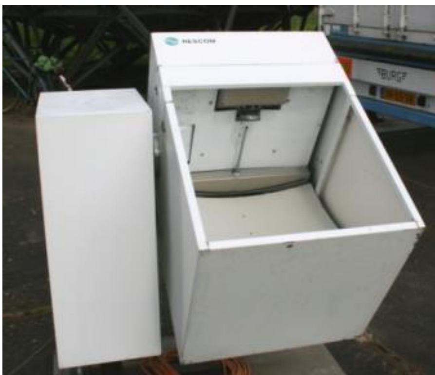
Figure 3.12: The RESCOM MWR installed at Cabauw remote sensing site
