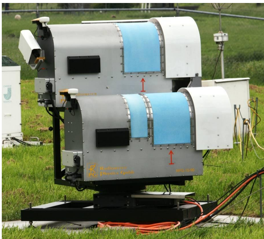
Figure 3.14: The ATPROP MWR installed at Cabauw remote sensing site
