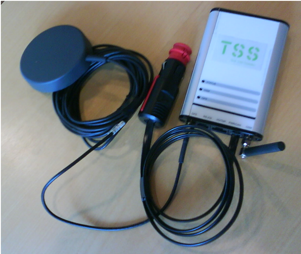
Figure 3.1 The GPS equipment. The logger is contained in a box with antenna for gprs communication (short stick mounted to the right). It is powered via a connector plug for 12 V outlet ((black/red in the middle) and supported with a GPS antenna with a magnetic holder for car roof mounting (blue “puck” to the left).
