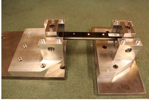
Figure 44: *HCF fixture with attached test specimen.*
