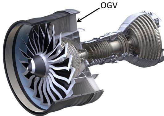
Figure 1: *GEnx engine with position of OGV indicated.*
