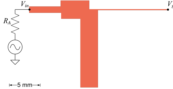
Figure 2.11: Layout of the RF voltage transformer metal pattern on PCB.
