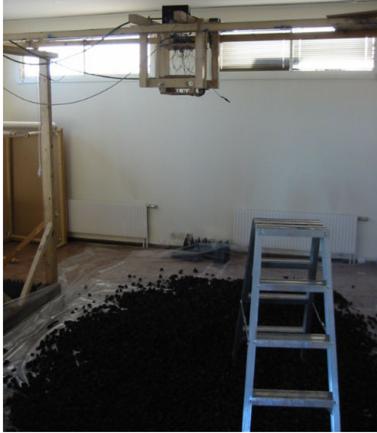
Figure 3.9: The laboratory imaging experiment setup, in this case with coke spread on the floor. The interferometer array is found at the top center of the image.
