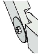
The bridge meets ground in tracks that allow movement
