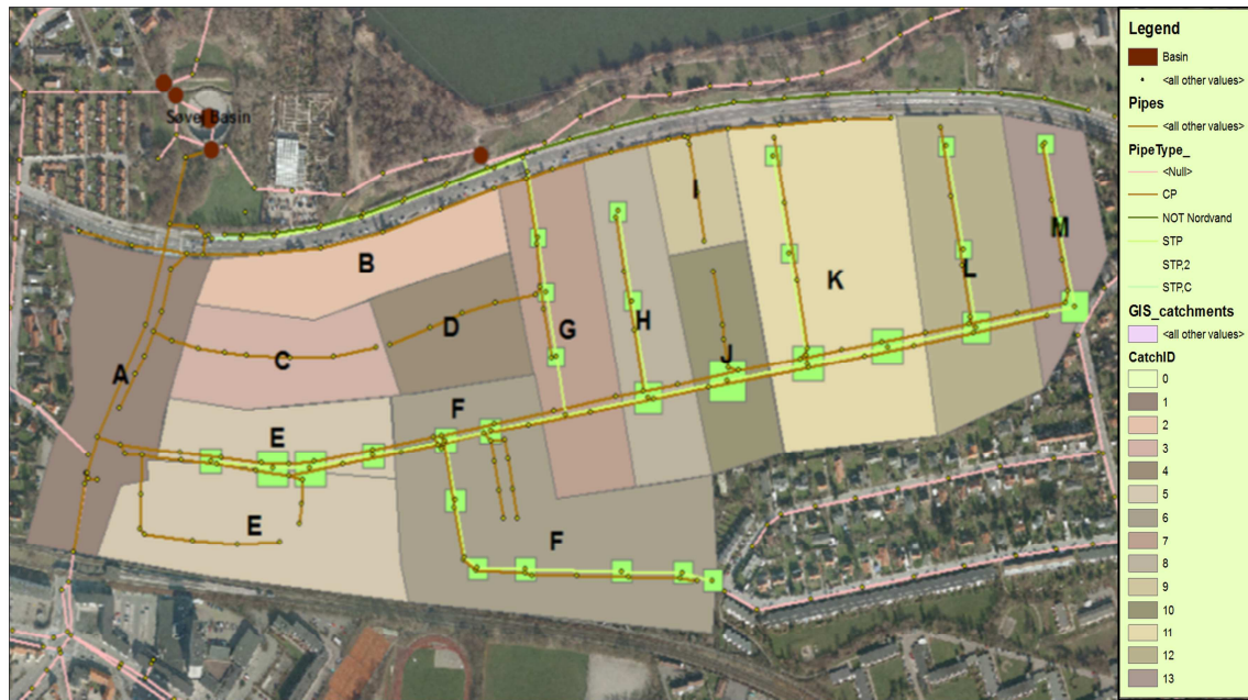
Figure 20, sewerage system in the current situation, (separated pipes and catchments are green)
