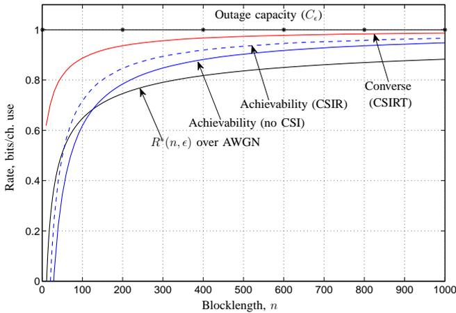
Fig. 2. Achievability and converse bounds for the quasi-static SIMO Rician-fading channel with  $K$ -factor equal to 20 dB, two receive antennas, SNR =  $-1.55$  dB, and  $\epsilon = 10^{-3}$ .
