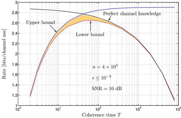
Fig. 1. Achievability and converse bounds for the block-fading Rayleigh-fading channel with no a priori CSI available at the transmitter and at the receiver;  $n = 4 \times 10^4$ , SNR = 10 dB, and  $\epsilon = 10^{-3}$ .
