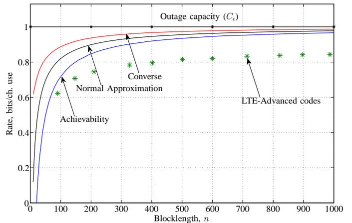
Fig. 3. Comparison between achievability and converse bounds and rate achievable with the coding schemes in LTE-Advanced. We consider a quasi-static SIMO Rician-fading channel with  $K$ -factor equal to 20 dB, two receive antennas, SNR =  $-1.55$  dB,  $\epsilon = 10^{-3}$ , and receive CSI. The star-shaped markers indicate the rates achievable by the turbo codes in LTE-Advanced (QPSK modulation and ten iterations of a max-log-MAP decoder [15]).
