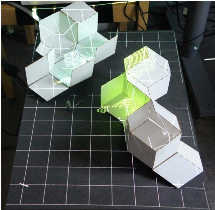
Fig. 10 shows the result of a small buildup. The two conglomerates are in balance over the single initial building block. They each attempt to create shade and reflect light onto the respective areas where the light sensors are placed.
