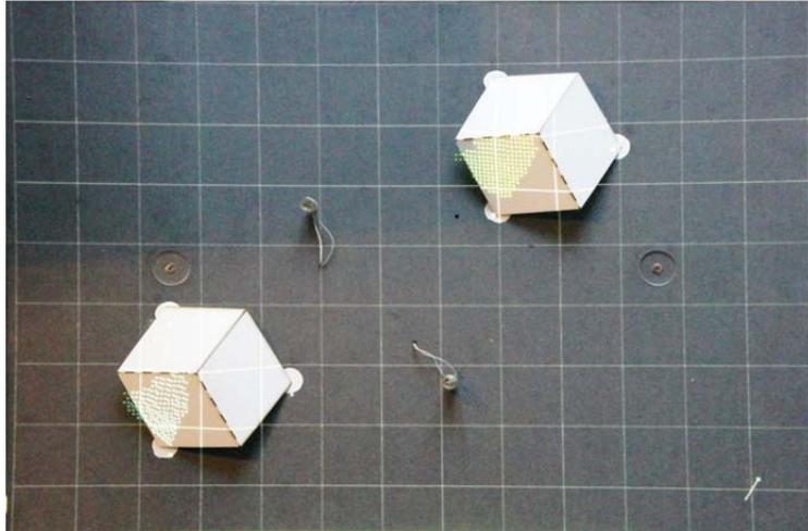
Fig. 8; Pressure sensors are placed in the baseplate under each footing of the start blocks. Two light sensors are placed next to each start point and two air flow sensors are placed between the start blocks. The conglomerates are monitored from the top by a Kinect Xbox 360 3d sensor, and a projector is placed right behind it to project on the building blocks where to add further blocks.
