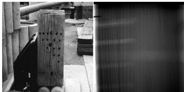
Figure 3.5 Simulated deterioration that caused the loss of cross-section resulted in a deviation in the greyscale on the X-ray image (N.C.P.T.T., 2005).
