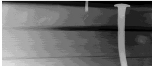
Figure 3.3 Deterioration of the metal fastener due to corrosion in the shrinkage crack of the beam.
