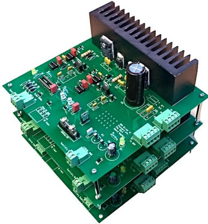
Figure 5.4: Three power converter boards
