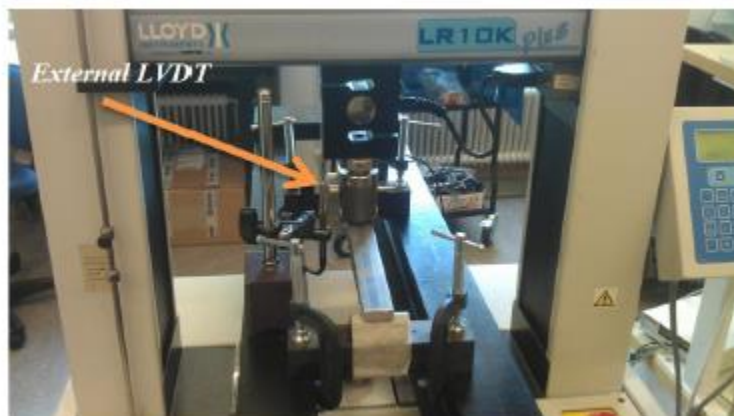
Figure 24 TRB specimen being tested
