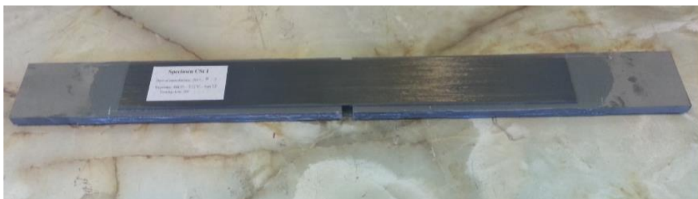
Figure 29 DLS specimen curing
