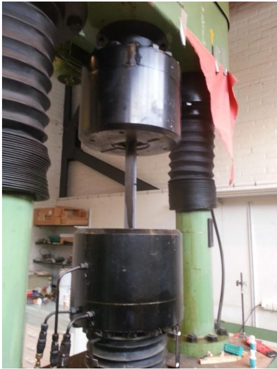
Figure 30 DLS specimen being pulled
