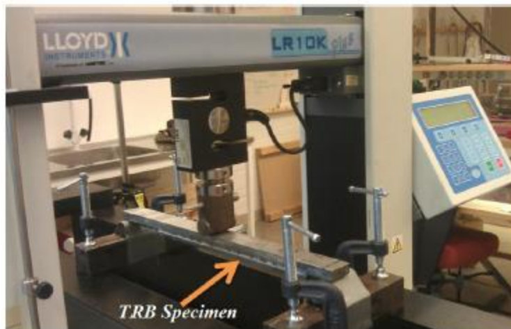
Figure 23 TRB specimen being tested
