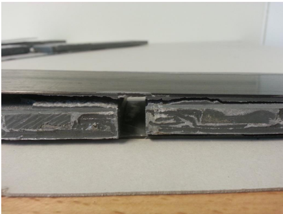
Figure 32 Cohesive failure in the specimens
