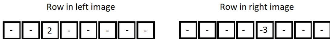
**Figure 41:** Two rows of disparities from different images. The ‘-’ means that the pixel does not have any valid disparity.
