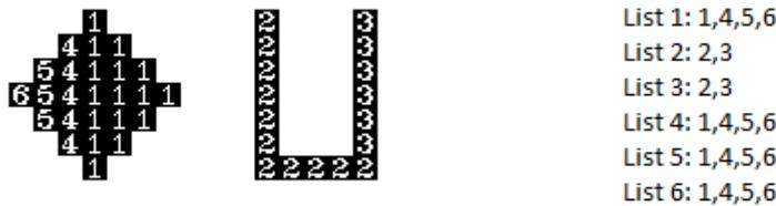
**Figure 15:** Here is an image with two components (a rhombus and a U) and the belonging list of connected labels. The number in each pixel is the label assigned to the pixel in the first pass. The image is traversed from top left corner.
