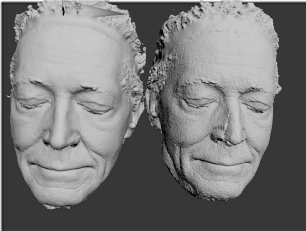
**Figure 46:** *The above image displays two meshes. The mesh to the right has been created without any sub-pixel disparities or refinement, and it is very apparent with the discrete levels on the surface. The left image has been refined with both a photometric and smoothness term. The dataset used to create the above meshes was given by Beeler et al. (Beeler et al., 2010).*
