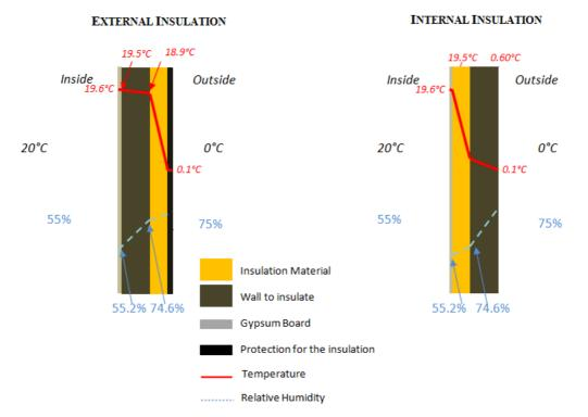
box", the thermal bridges are suppressed (Plouget). The choice of the type of insulation depends on every project.
