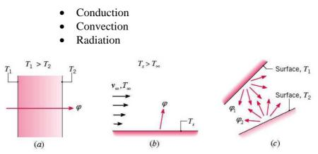
*Figure 2.1 Illustration of the modes of heat transfer: a) conduction, b) convection, c) radiation (Ghiaus and Brau 2011)*
