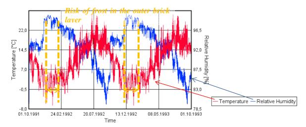
Figure 5.4 Temperature and relative humidity in the outer brick façade
