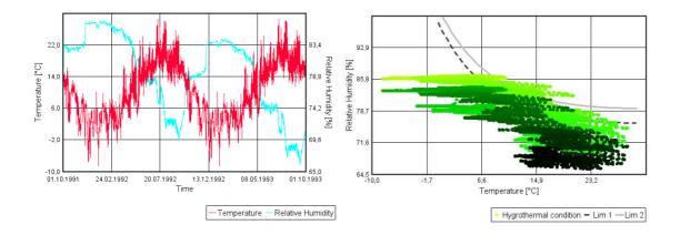
*Figure 5.11 Temperature and relative humidity in the outer brick layer.*
