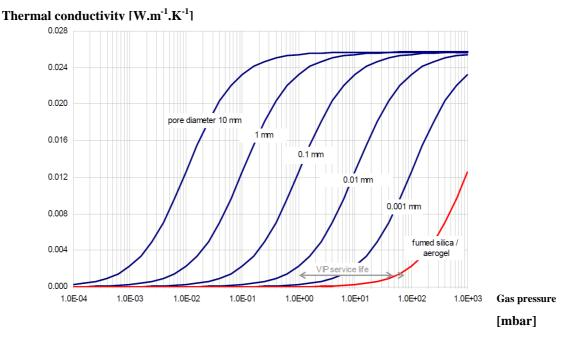
*Figure 3.3 Thermal Conductivity of air due to gas conductivity as a function of pore diameter (Simmler et al. 2005)*
