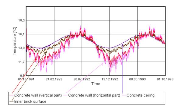
Figure 5.2 Temperature on the surface for the different materials
