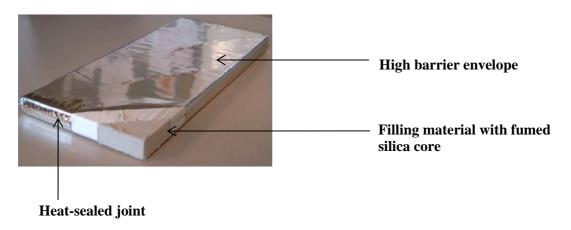
Figure 1.2 Example of vacuum insulation panel (Tenpierik 2009)
