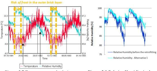
Figure 5.7 Temperature and relative humidity in the outer brick façade
