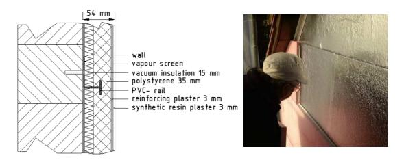
Figure 3.6 VIPs for an external insulation, Germany. On the left, a cross section of the facade. On the right, during the installation (Binz et al. 2005)
