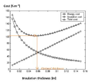
Figure 6.2 Variation of cost with insulation thickness (Ozel 2012)
