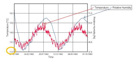
Figure 5.5 Temperature and relative humidity in the inner brick façade
