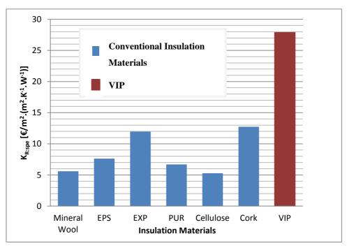
Figure 3.10 Values of the cost per thermal transmittance for different materials.
