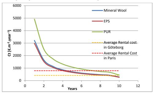
Figure 4.15 Minimal required annual rent to pay back the extra-cost of an insulation with VIPs.
