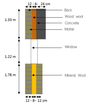
Figure 4.6 presents a cross-section of the façade before the retrofitting.
