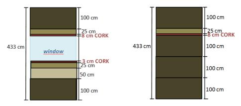
Figure 4.9 Layout of the VIPs. On the left, layout for the part of the facade with windows. On the right, layout for the opaque facade
