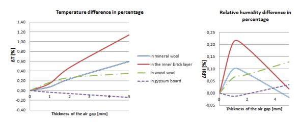
Figure 5.18 Influence of the air gap on the temperature and relative humidity in percentage
