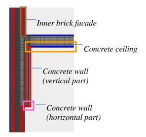
Figure 5.1 Location of the surface where the surface temperatures have been calculate
