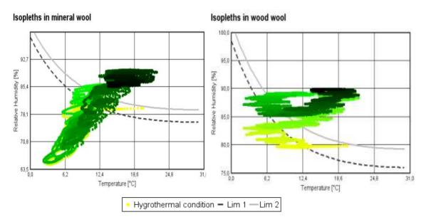
Figure 5.6 Risk of mould growth in the insulation materials
