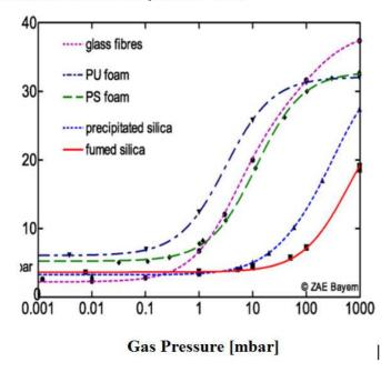
Figure 3.4 Thermal conductivity of several porous materials as a function of gas pressure at 20°C (Simmler et al. 2005)
