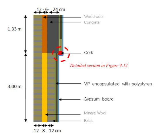
Figure 4.8 Solution for the retrofitting of the façade – Vertical projection
