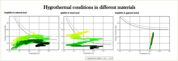
Figure 5.13 Isopleths in different materials (the lightest colours represent the conditions in the start of the calculation time whereas the darkest colours represent the end of the calculation)
