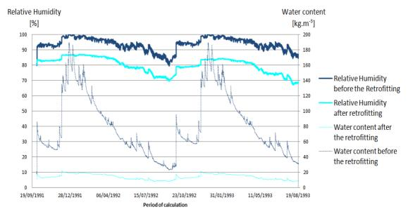
Figure 5.10 Effects of the retrofitting on relative humidity and the water content in the outer brick layer
