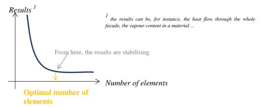
Figure 6.1 Proposition to find the optimal number of elements for the grid in WUFI 2D.
