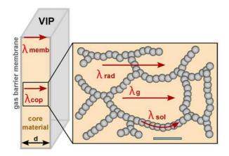
Figure 3.2 Heat transfer through a VIP: influence of the different thermal conductivities (adapted from Bouquerel et al. 2012a)
