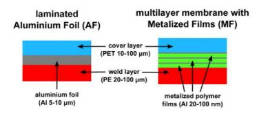
*Figure 3.1 Design of VIPs envelope: Aluminium Foil and Metalized Films (Bouquerel et al. 2012a)*
