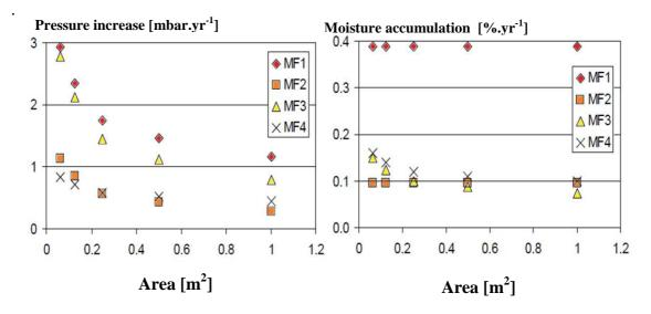
*Figure 3.5 Moisture accumulation and pressure increase in VIP with MF envelope* (23 °C, 50% RH, 1bar) (Simmler et al. 2005)
