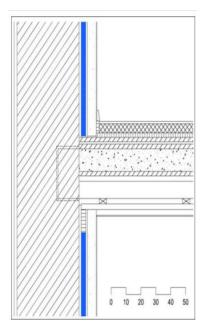
Wall Structure:External rendering, existing: 20mmQuarry Stone wall, existing: 430mmInterior plaster, existing: 15 mmVIP, new: 30 mm (in blue)Air gap: 10 mmSolid Gypsum board, new: 60 mmInterior plaster, new: 5 mm
