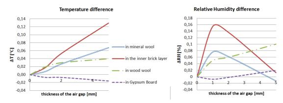
Figure 5.17 Influence of the air gap on the temperature and relative humidity
