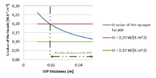
Figure 4.11 U value of the opaque facade
