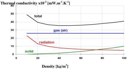
Figure 2.3 Heat transfer in conventional insulation materials (Simmler et al. 2005)
