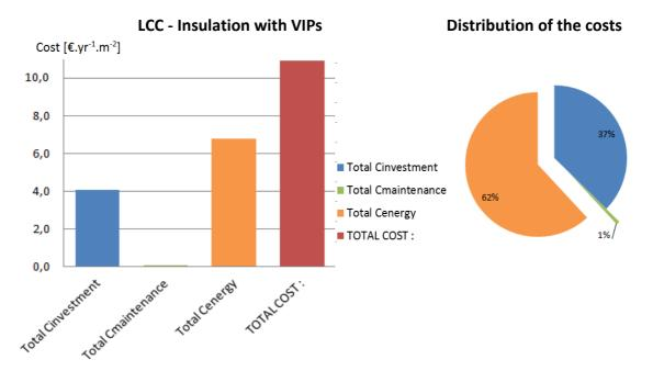
*Figure 4.13 Results for LCC with an insulation system with VIPs (N=50 years)*
