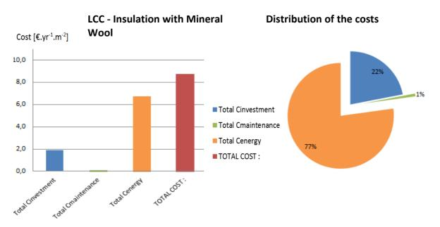
*Figure 4.14 Results of LCC with a mineral wool insulation (N=50 years)*
