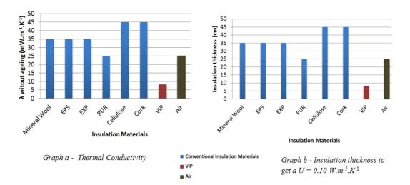
*Figure 2.2 Thermal properties of Insulation Materials (adapted from the values from Jelle 2011)*
