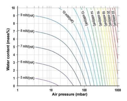
Figure 3.9 Thermal conductivity of fumed silica as a function of air pressure and water content, at external pressure of 1 bar and external temperature  $20 \, {}^{\circ}C$  (Baetens et al. 2009)
