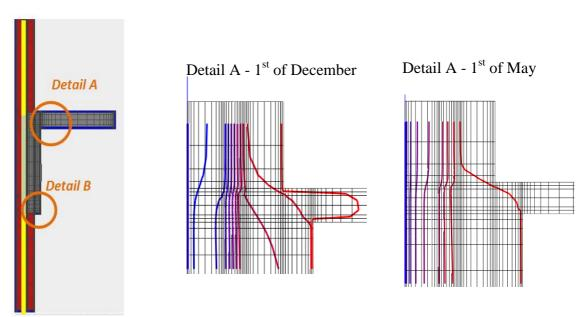
Figure 5.3 Study of the thermal bridges effects in the façade before the retrofitting
