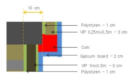
Figure 4.12 Detailed Section of the retrofitted facade
