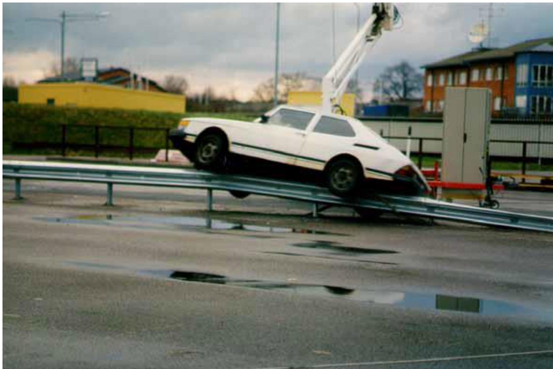
Picture 14 Consequences of a collision when using a down turned end terminal barrier (Wenäll, 2006).
