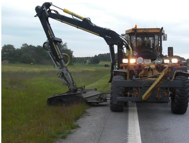
Picture 2 Illustration of the machinery work when mowing alongside a road (Karim, 2012).
