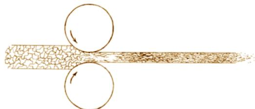
Figure 2.2 Cold rolling process of a steel plate
