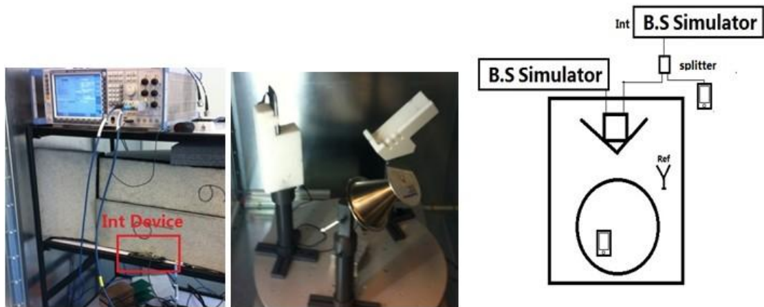
Figure 4. 2 The Configuration and scheme of inter-cell Co-channel interference based on WCDMA standard
