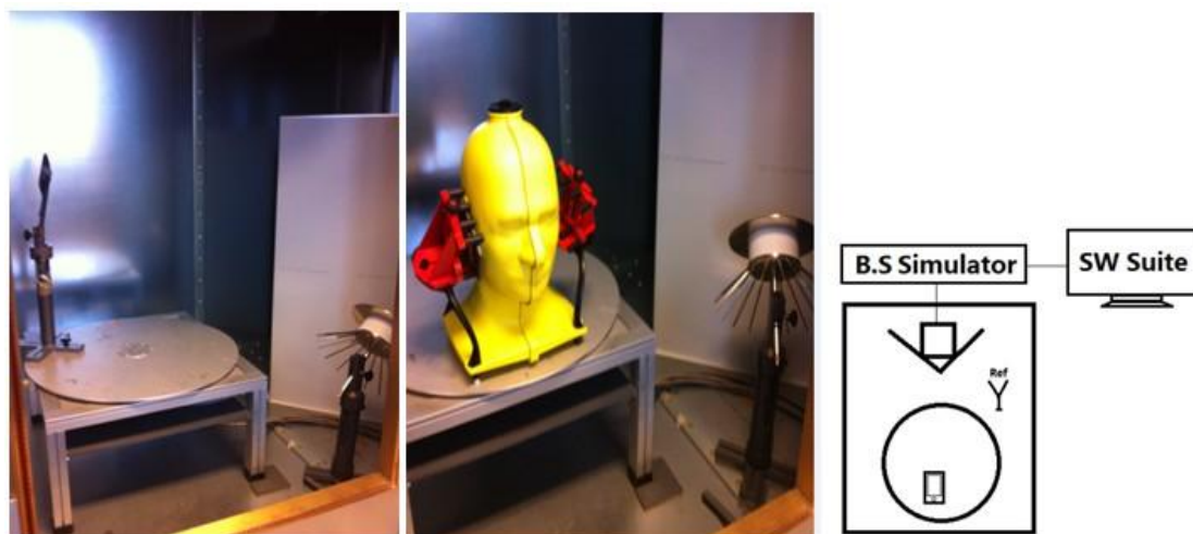
Figure 3. 7 Configuration and scheme of TRP measurement, set up for WCDMA measurement (left); testing TRP value of WCDMA with phantom (middle)
