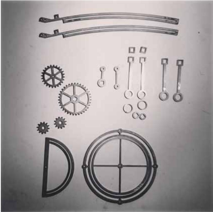
Optical Instrument - Laser cut parts
