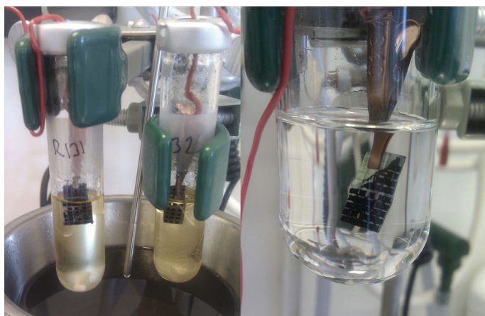
Figure 58. Left picture shows the reaction setup (after reaction) and right picture shows the cleaning setup, performed three times for a minimum of 1 h after every reaction step.
