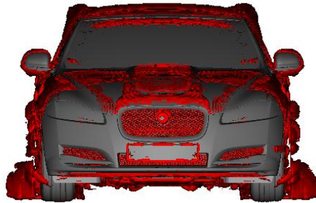
Figure A-6 Isosurfaces of Q greater than 3000 (MRF)
