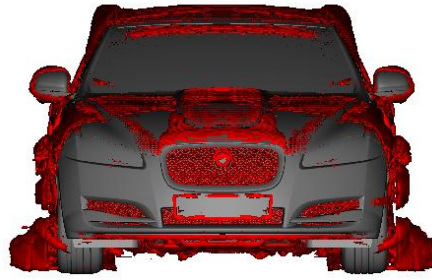
Figure A-5 Isosurfaces of Q greater than 3000 (Sliding Mesh)
