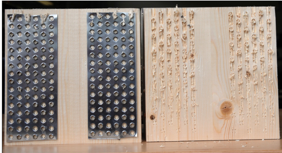
Figure 3.7 Test specimen with strips of punched-out holes before the test (left) and after the test (right). Photo taken from (SP 2012)
