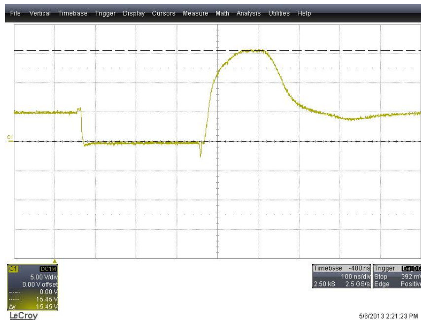
Fig. 5.14 V_{out} versus time where t_{on} = 4.4 \cdot 66ns = 290ns and Z_L = 50\Omega .
