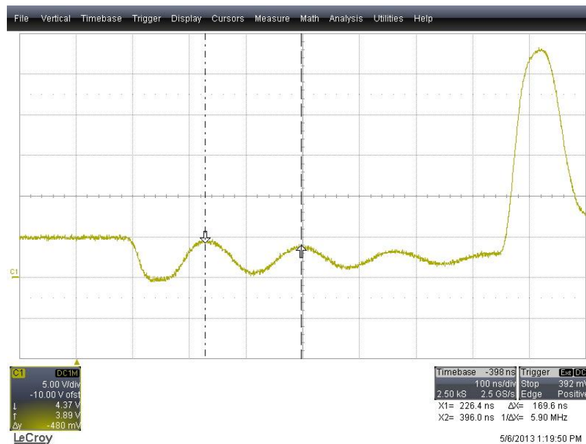
Fig. 5.10 Voltage at the middle of the LTL for the same modulation pattern as in Figure 5.9. Z_L = 61\Omega .
