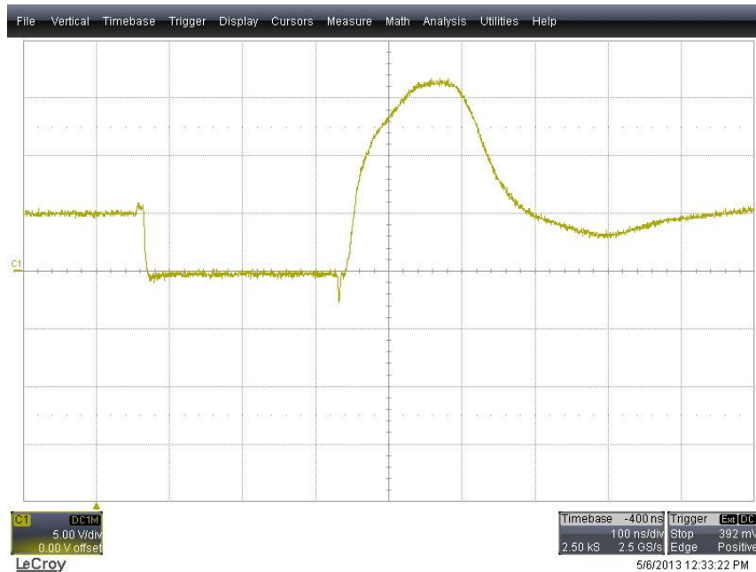
Fig. 5.8 V_{out} versus time where t_{on} = 4 \cdot 66ns = 264ns and Z_L = 61\Omega .
