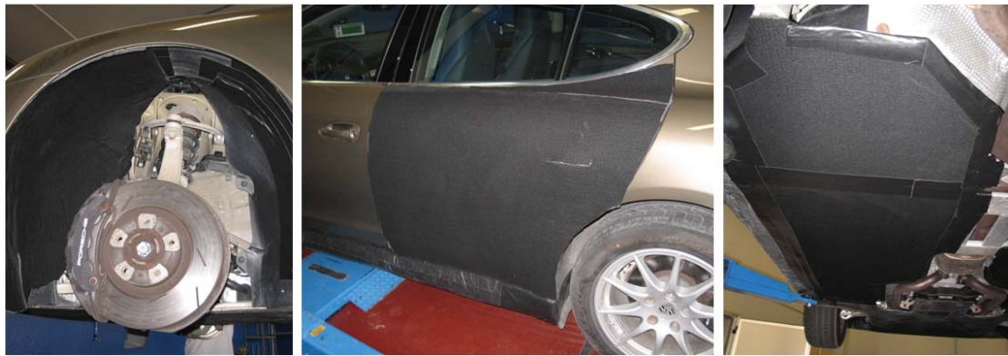
Fig. 2.6. The test vehicle masked with fleece.
