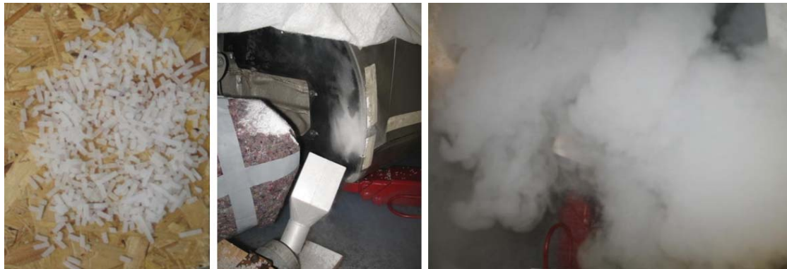
Fig. 3.32. The CO 2 pellets and the electric blower.
