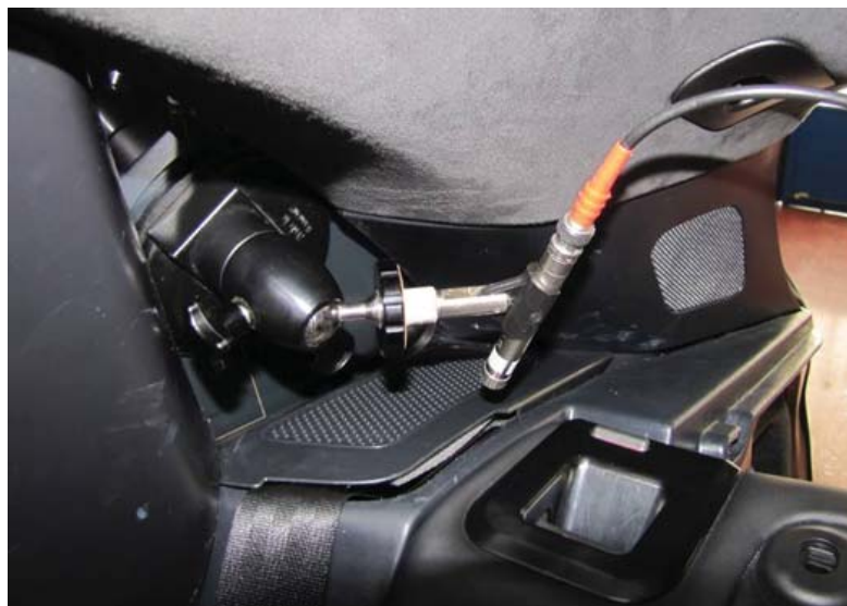
Fig. 4.9. The seatbelt outlet with attached microphone.
