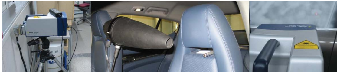
Fig. 3.13. Laser-Doppler-Vibrometer test setup.
