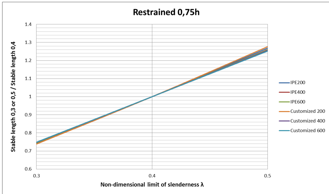
Figure 43 The stable length for a restrained beam at 0,75h , assuming different non-dimensional limit of slenderness.
