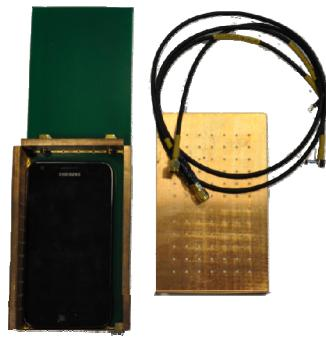
Figure 7. One of the reference antennas used for the measurements presented in this paper. An RF enclosure is attached to the antennas, in which the handset used as demodulator is inserted. This will assure shielding of the handset antennas and of device noise coupled to the reference antenna. The device receivers are connected to the reference antenna by short RF cables.
