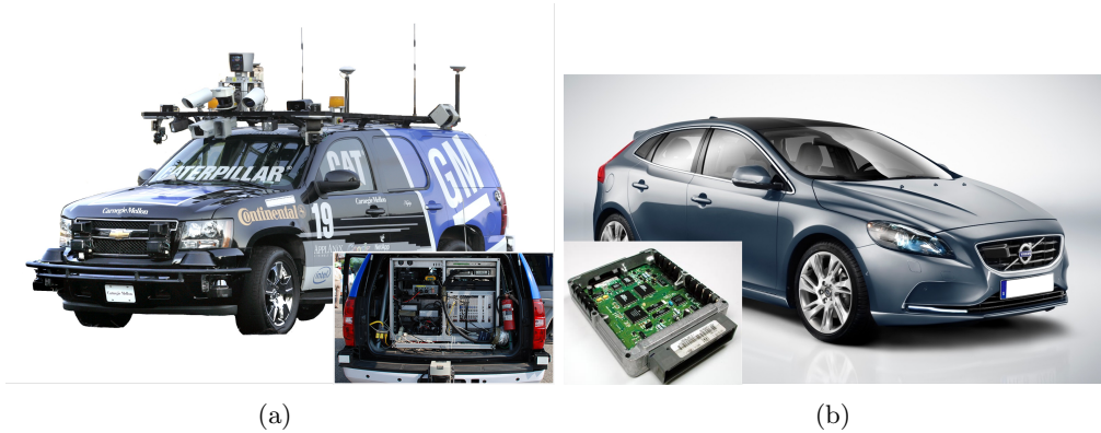
Figure 1.1: 1.1(a) University of Carnegie Mellon’s entry to the DARPA Urban Challenge. 1.1(b) Volvo V40 with a sample electronic control unit. Such unit typically hosts several functions running on sub-gigahertz processor and with allotted memory in the kilobyte range.
