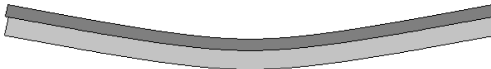
Figure 7.12 Assumed interaction between beam and slab when the new load is added.
