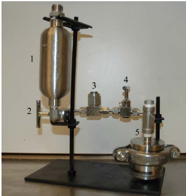
Figure 3-1 Solubility measurement equipment. 1 – Sample vessel 2,4 – Valves 3 – Filter housing 5 –Filtrate container. Picture adapted from Gourdon (2009a).
