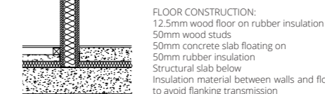
DETAIL 1:20 Isolating wall between the big and small rehearsal rooms
