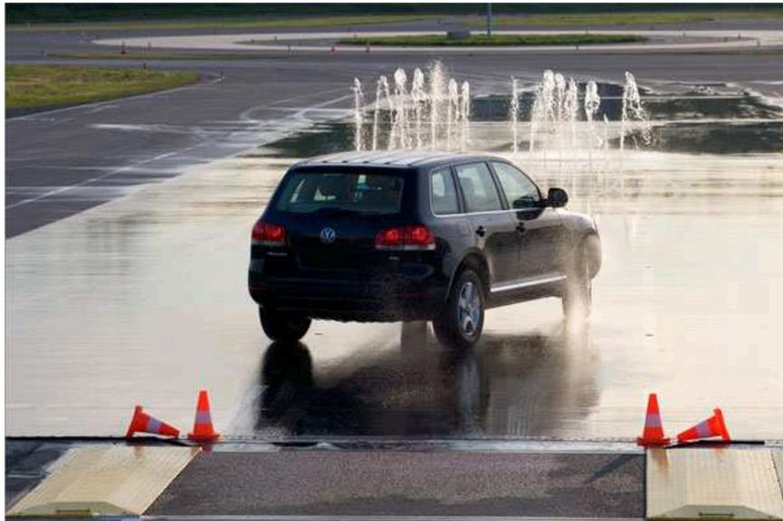
Figure 6.5: Destabilize a car using kick plate (low friction surface designed after the kick) [101].
