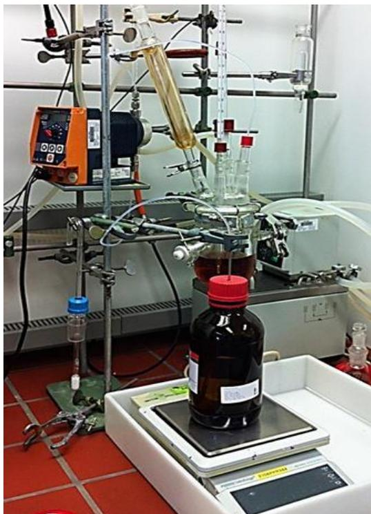
Figure 9 Instrumental set-up for the cyanoethylation reaction.
