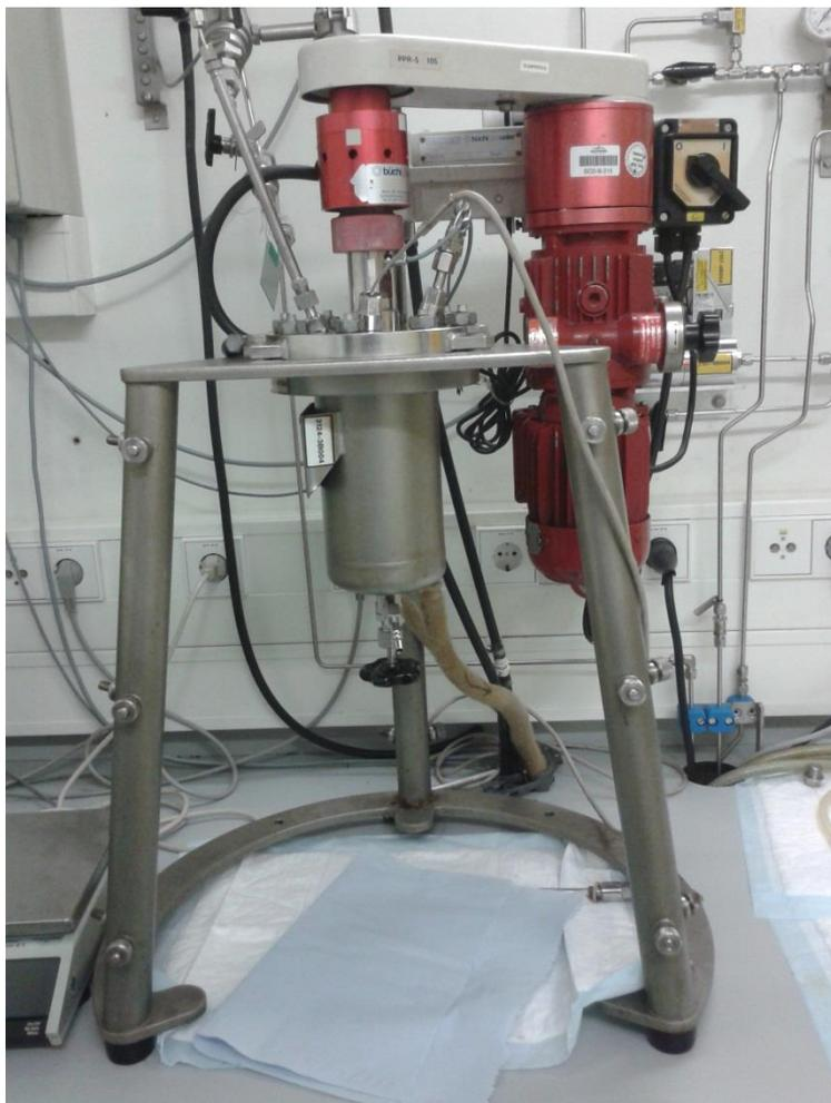
*Figur 10 High temperature and high pressure in an autoclave used in the hydrogenation.*
