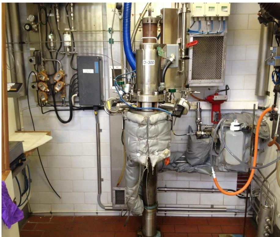
Figure 8 autoclave used in the polymerization of ethylene oxide.
