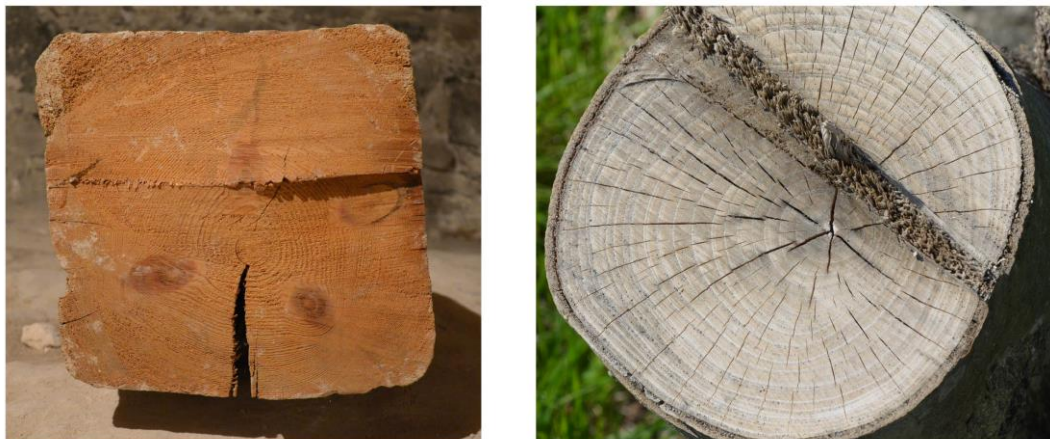
Figure 2.5 Cross-section of a removed timber part from Skansen Lejonet showing dense annular rings (Left), cross-section of a young tree with fast growth (Right).
