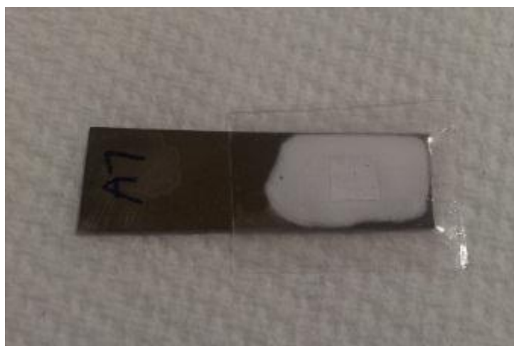
Figure 21: Sol-gel made form base-catalyzed hydrolysis in an ammonia atmosphere.
