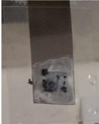
Figure 18: Too much deposition in relation to zeolite thickness and dendrites are seen to start forming.
