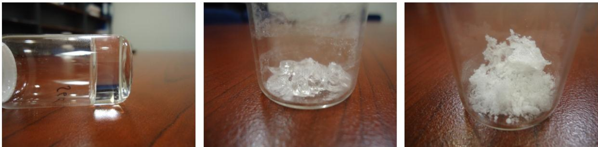
Figure 19: Bulk sol-gel. Left: After gelation. Middle: After room temperature drying. Right: After freeze-drying. Neither drying method gave good results and attempts were more focused on thin-film sol-gel instead.
