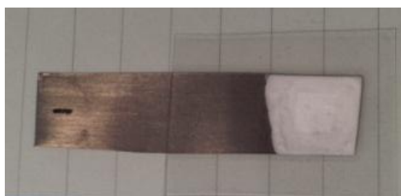
Figure 8: Titanium electrode with a white zeolite layer in the bottom
