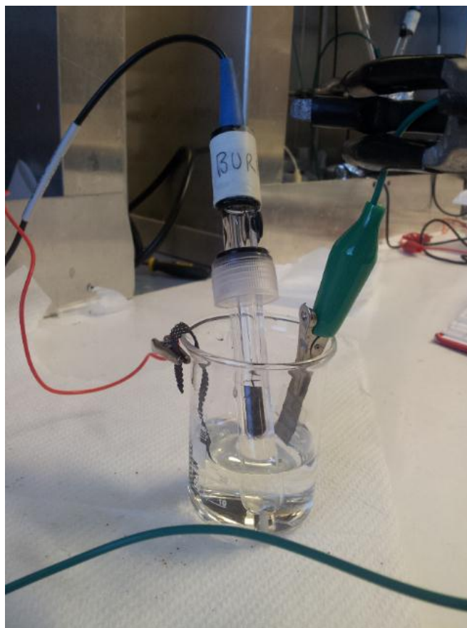
Figure 2: Experimental setup for the cycling experiments. The green cable is connected to the working electrode, the red cable is connected to the counter electrode, and the vial in the middle is the SCE reference electrode
