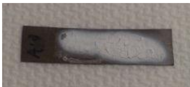
Figure 23: Base-catalyzed sol-gel with cracks
