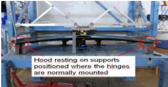
Figure 2.7.4– Constraints setup for hinges, provided by Christian Forsberg, Design Engineer, Autoliv.
