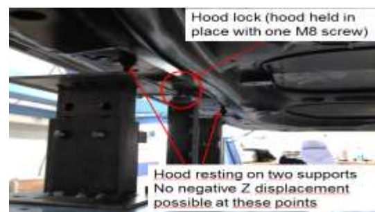
Figure 2.7.3– Constraints setup for latch and regulators, provided by Christian Forsberg, Design Engineer, Autoliv.
