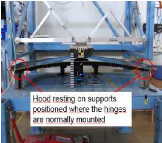
Figure 7.5.3- Constraints of rear part, provided by Christian Forsberg, Autoliv.
