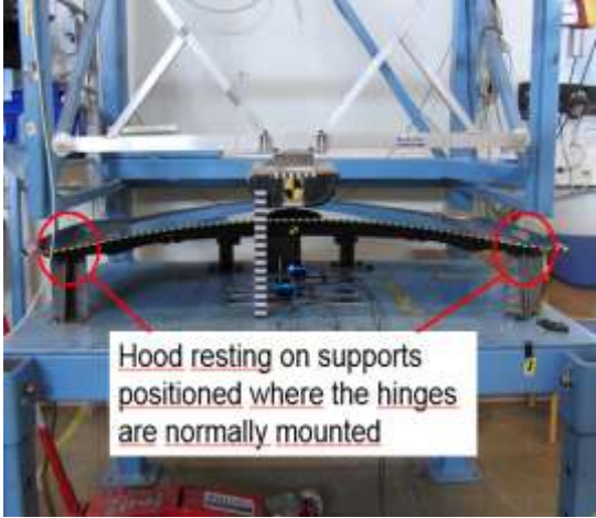
Figure 7.5.7- Constraints of rear part, provided by Christian Forsberg, Autoliv.
