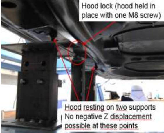
Figure 7.5.2- Constraints of front part, provided by Christian Forsberg, Autoliv.
