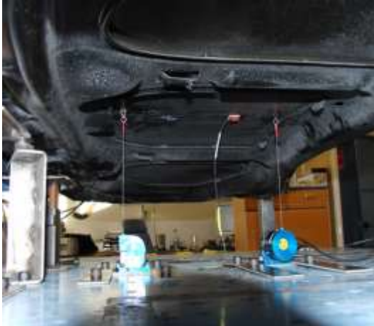
Figure 7.5.4- Wire sensor/Stringpot for rear edge alignment, provided by Christian Forsberg, Autoliv.
