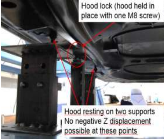
Figure 7.5.8- - Constraints of front part, provided by Christian Forsberg, Autoliv.
