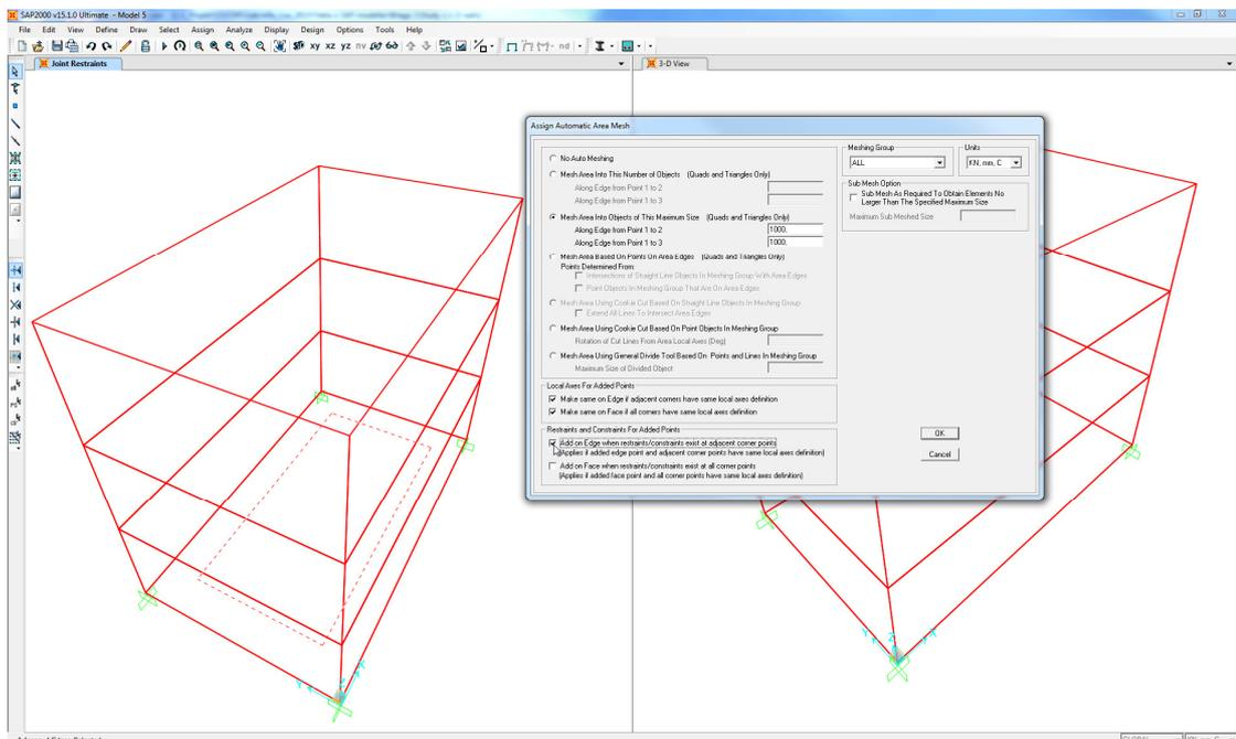
7. To apply a load to the model a new load pattern was created in the *Define Load Pattern* box.
