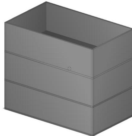
*Figure 3.7 A model with several panel and slab elements in connection to each other.*
