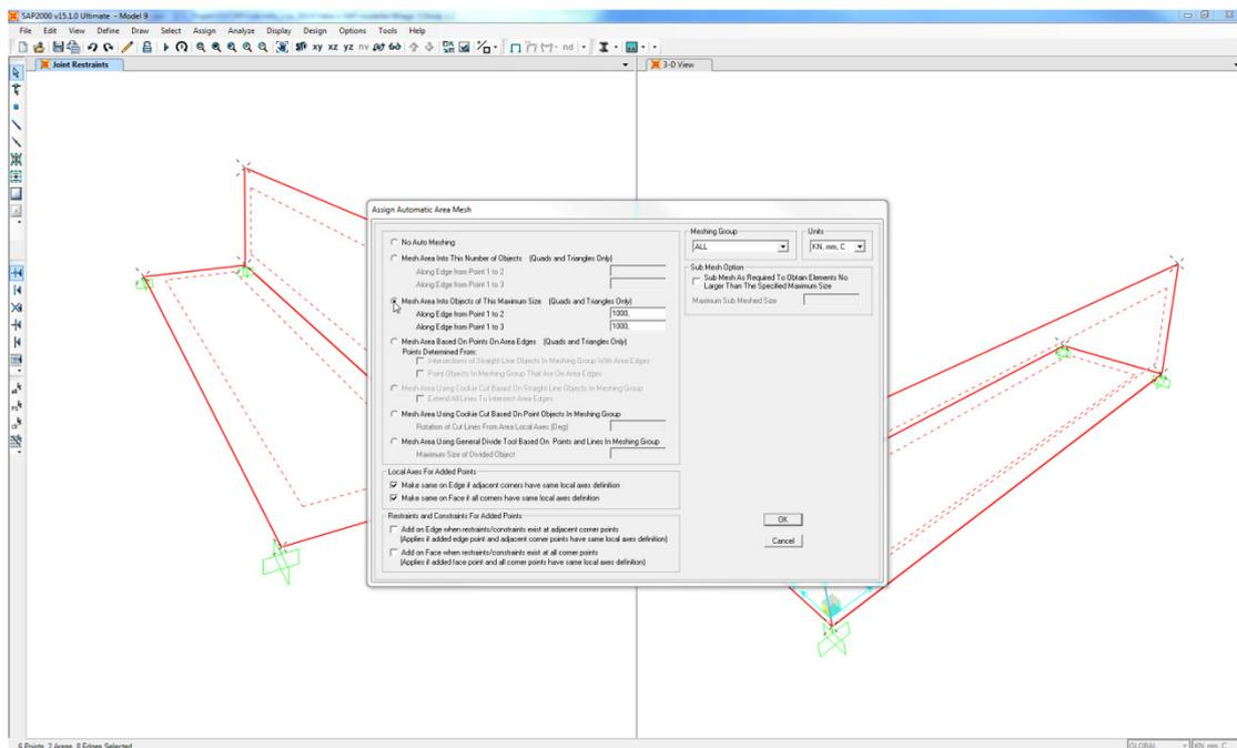
12. A linear static analysis was performed by the *Set Load Cases to Run* box. The MODAL case was set to *do not run* in order to save time. This was done for all further studies.
