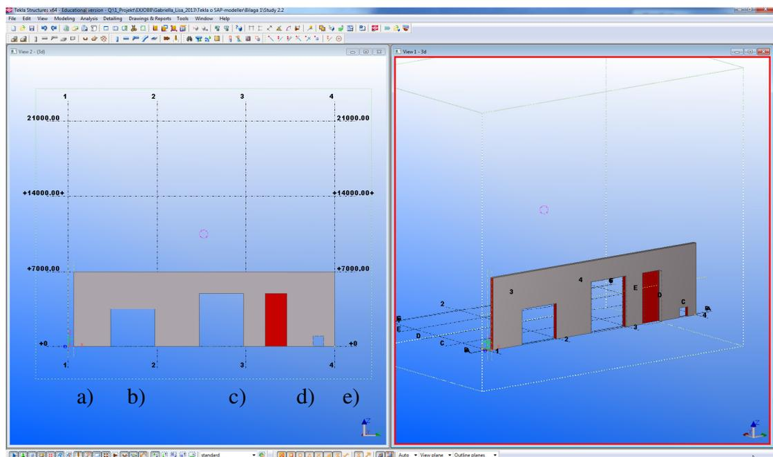
2. An *Analysis & Design model* was created. No analysis lines or nodes was generated for the *partly cut out*.
