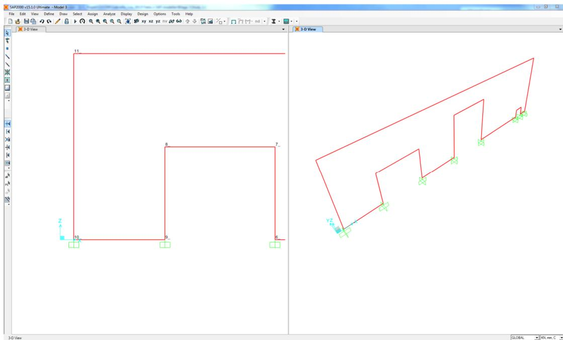
6. By opening the *Assign Automatic Area Mesh* box it could be seen that the program recommend the meshing option *Mesh Area Using General Divide Tools Based On Points and Lines In Meshing Group*. The maximum size of divided objects chosen by the program was kept.
