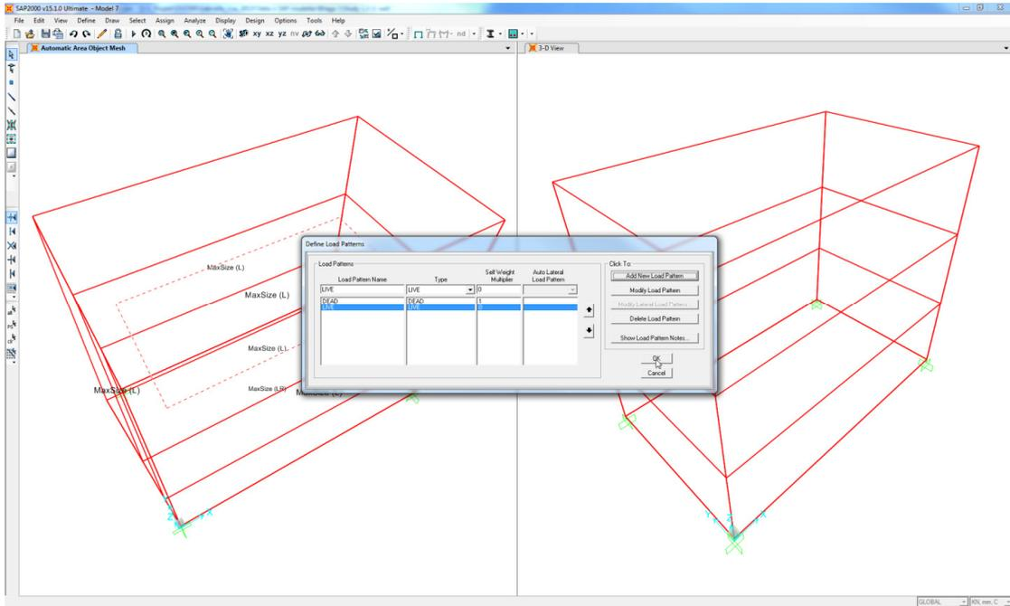
17. A *surface load* in the direction of the gravity (z-direction) was applied to the top slab of the model.
