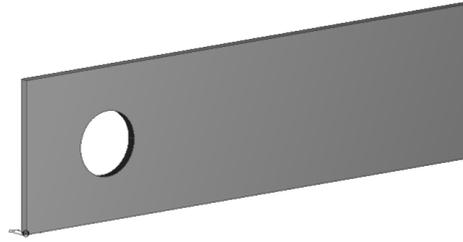
*Figure 3.26 A panel modelled in TS with a circular opening within the panel.*
