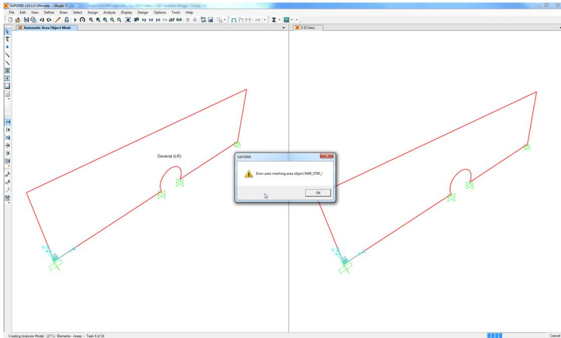
8. The meshing choice was changed to *Mesh Area Into Objects of This Maximum Size (Quads and Triangles Only)*. The maximum size chosen by the program was kept. In order to get a sufficient fine mesh the option *Sub Mesh As Required To Obtain Elements No Larger Than The Specified Maximum Size* was used and a maximum size of the elements were specified.
