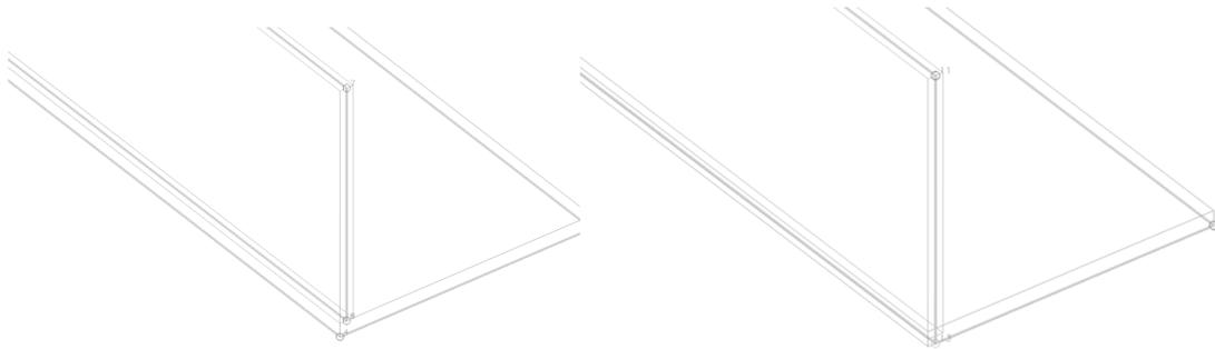
Figure 3.6 To the left: a model containing elements with not shared analysis lines. To the right: a model containing elements with shared analysis lines.
