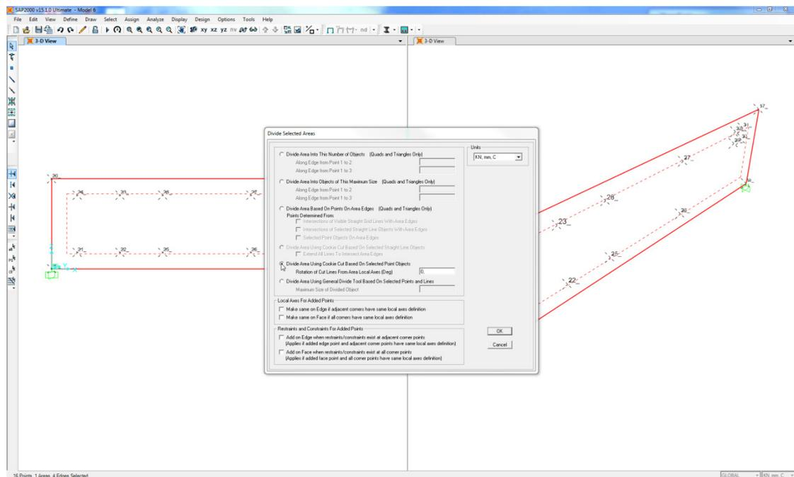
12. The model was divided into smaller areas based on the nodes inside the model.
