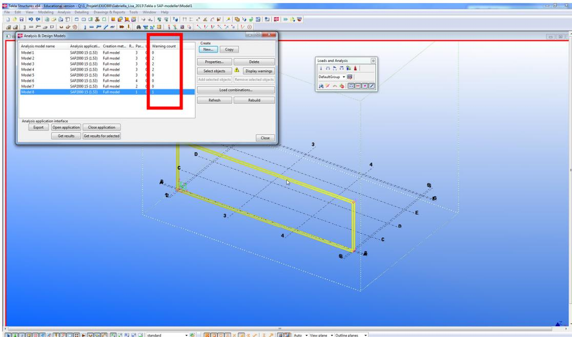
4. To get detailed information about the *warning counts* the function *Display warnings* was used and the *warning counts* for the analysis was defined as “*Analysis element warning(s)*”.
