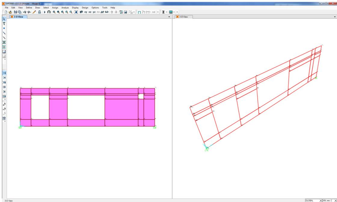
14. All nodes along the bottom edge of the slab were fully restrained.
