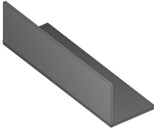
*Figure 3.5 A panel element in connection to a slab element modelled in TS.*
