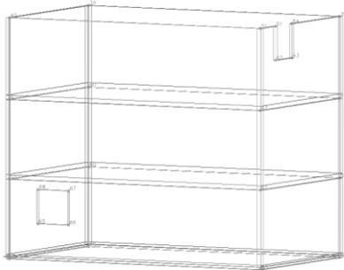
Figure 3.24 Created Analysis & Design model in TS for several panels containing opening.
