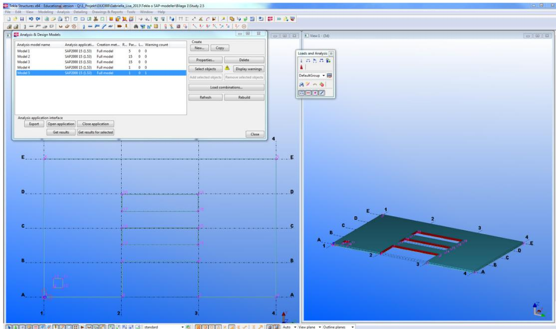
3. The *Export*-link was used. The result of the export was similar to the one concerning a panel containing openings. The opening at the edge of the slab were exported while the openings within the slab not were transferred. For the openings in the slab only the nodes were exported.
