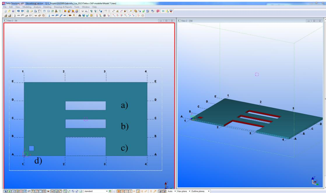
2. The *Analysis & Design model* was created. Analysis lines with nodes were generated for both the slab and each opening.
