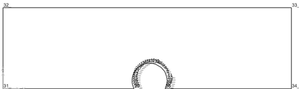
Figure 3.31 *The exported model for a panel element containing a circular opening at the edge.*
