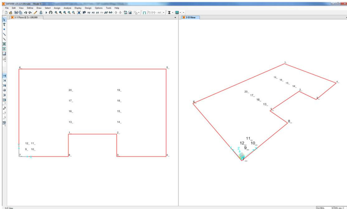
4. The model was divided into smaller areas in the *Divide Selected Area* box by choosing the option *Divide Area Using Cookie Cut Based On Selected Point Objects with the Rotation of Cut Lines From Area Local Axes*.
