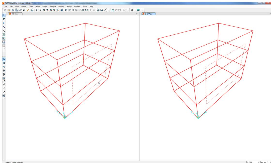
13. The corner nodes of the slab were fully restrained.
