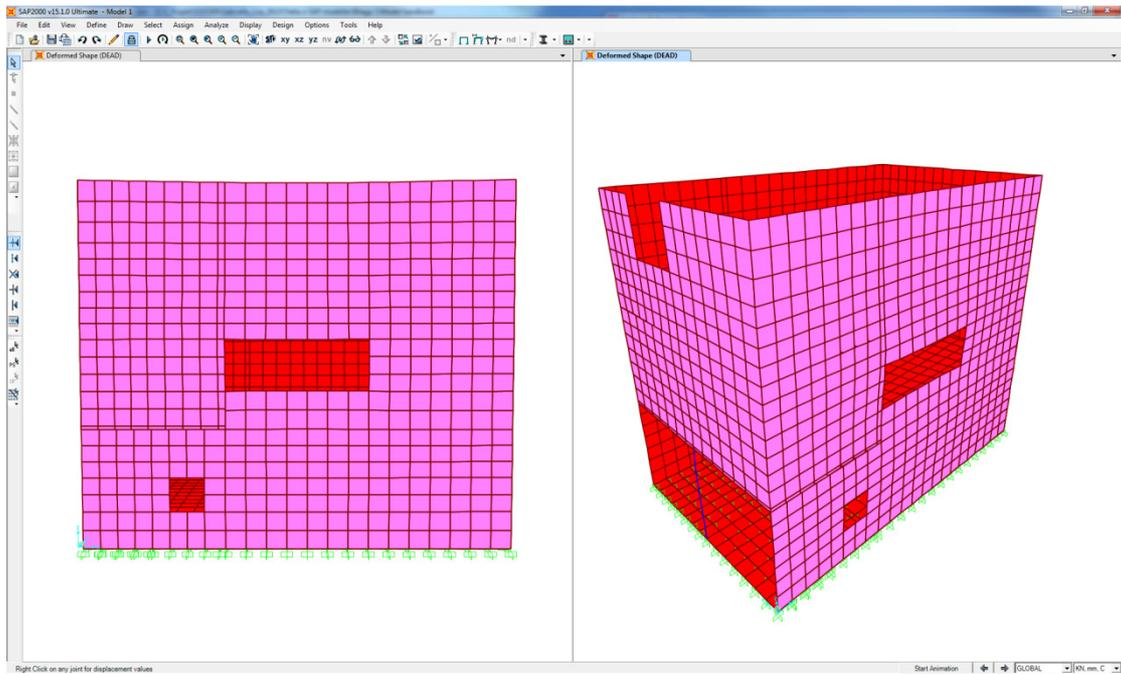
The model is analysed influenced only by dead weight and the result is displayed by a deformed shape. In order to get a more fine mesh the following steps can be included in the work (see next page).
