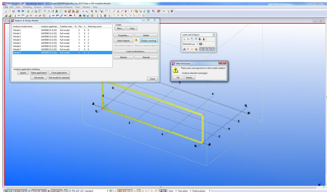
5. Further details about the warnings were displayed by the function *Details*. The report described that the panel was not fully connected or supported. In this case the *warning count* did not need to be fixed.
