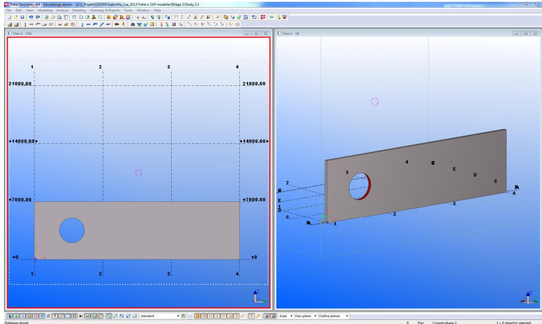
2. An *Analysis & Design model* was created. Analysis lines were created for both the panel and the circular opening.
