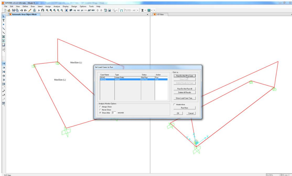
13. The model were meshed and restrains/constrains were generated at the corner of the slab. The slab was influenced only by the applied live load and it could be seen that the elements were deformed together and consequently was the panel and slab connected correctly.
