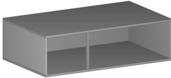
*Figure 3.36 The structure in TS containing panels and a column connected to the slabs.*
