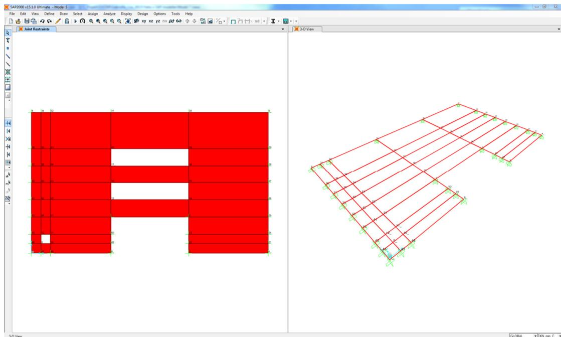
7. By opening the *Assign Automatic Area Mesh* box it could be seen that the program recommend the meshing option *No Auto Mesh*. The meshing option was changed to *Area Into Objects of This Maximum Size (Quads and Triangles Only)*. The maximum size chosen by the program was kept. In order to get a sufficient fine mesh the option *Sub Mesh As Required To Obtain Elements No Larger Than The Specified Maximum Size* was used and a maximum size of the elements was specified.
