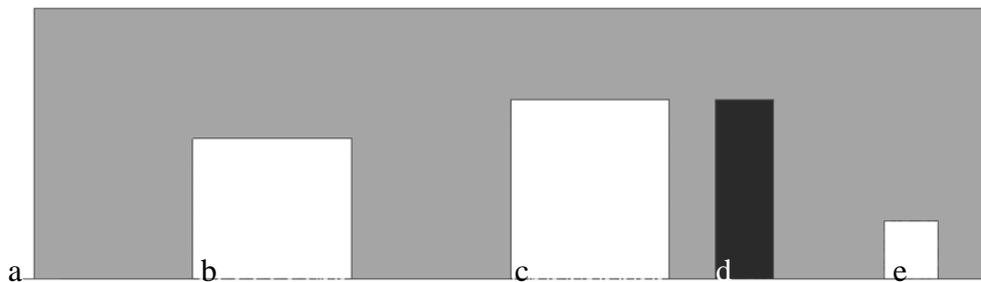
Figure 3.19 Openings modelled in a panel in TS, created with different modelling techniques.
