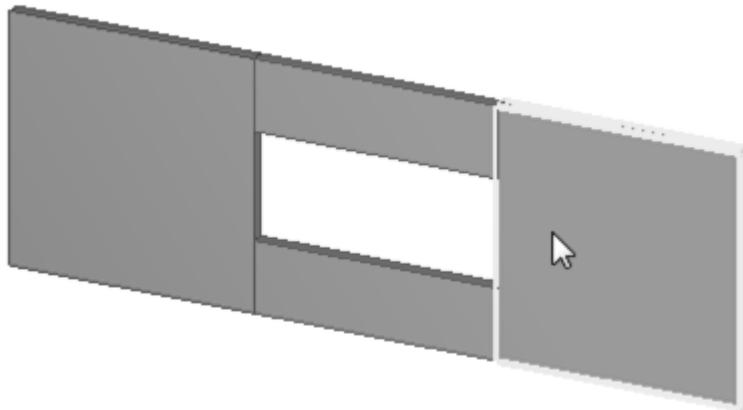
*Figure 3.15 Panels modelled to create an opening in the middle of the model.*
