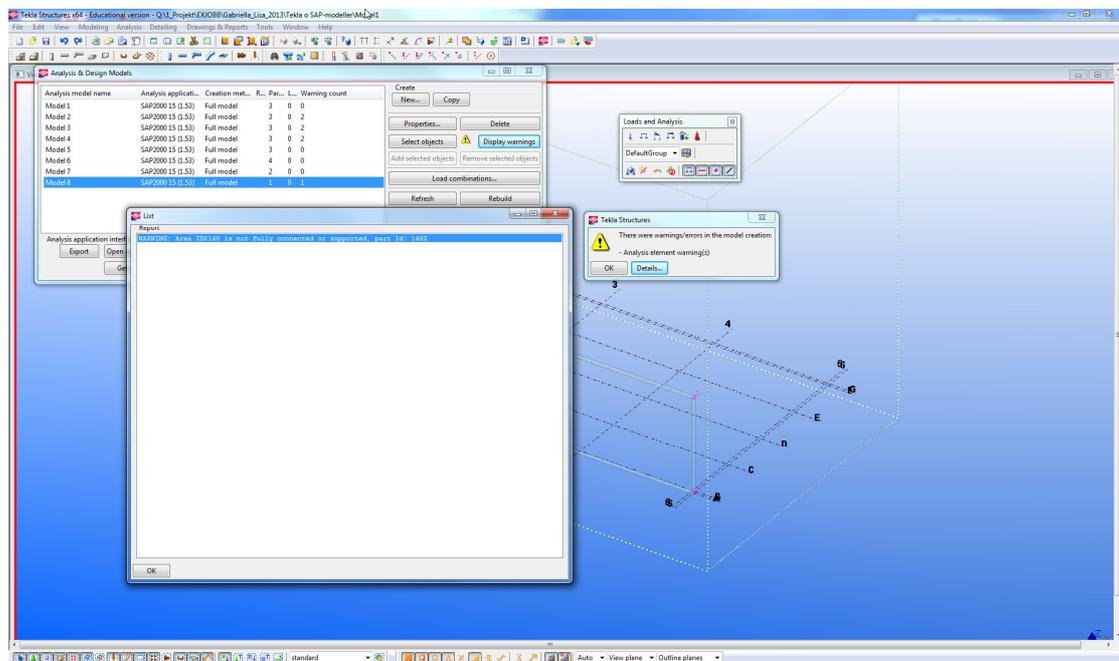
6. The *export* function was now used. A message appeared concerning creation of load combinations in TS. Since the loads should be applied by the structural engineer in SAP the option “No” was chosen. This message is a standard message that appears for every export if no load is applied in TS.
