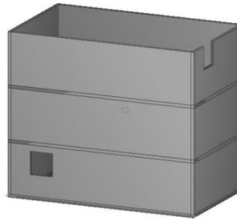
Figure 3.22 A model of several connected panel and slab elements containing openings
