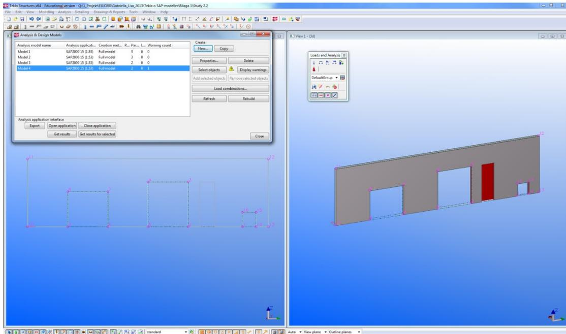
3. The model was exported to SAP. The openings at the edge of the panel were exported correctly independent of used modelling technique.
