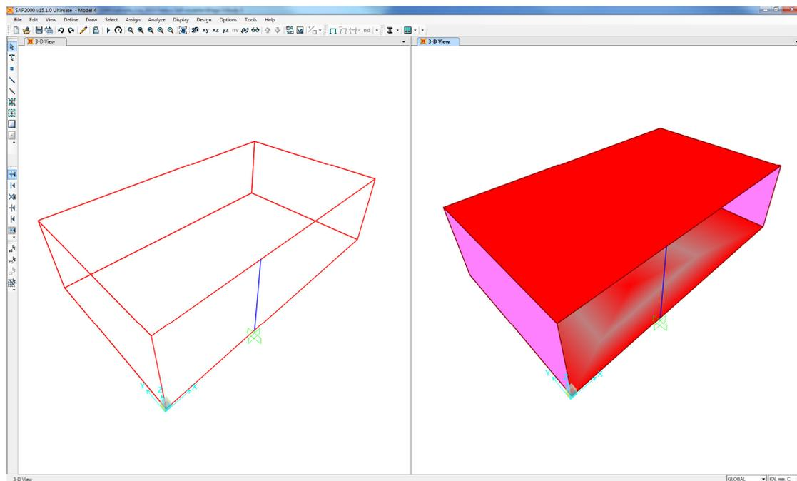
3. The corner nodes of the slab were fully restrained, including the node under the column.
