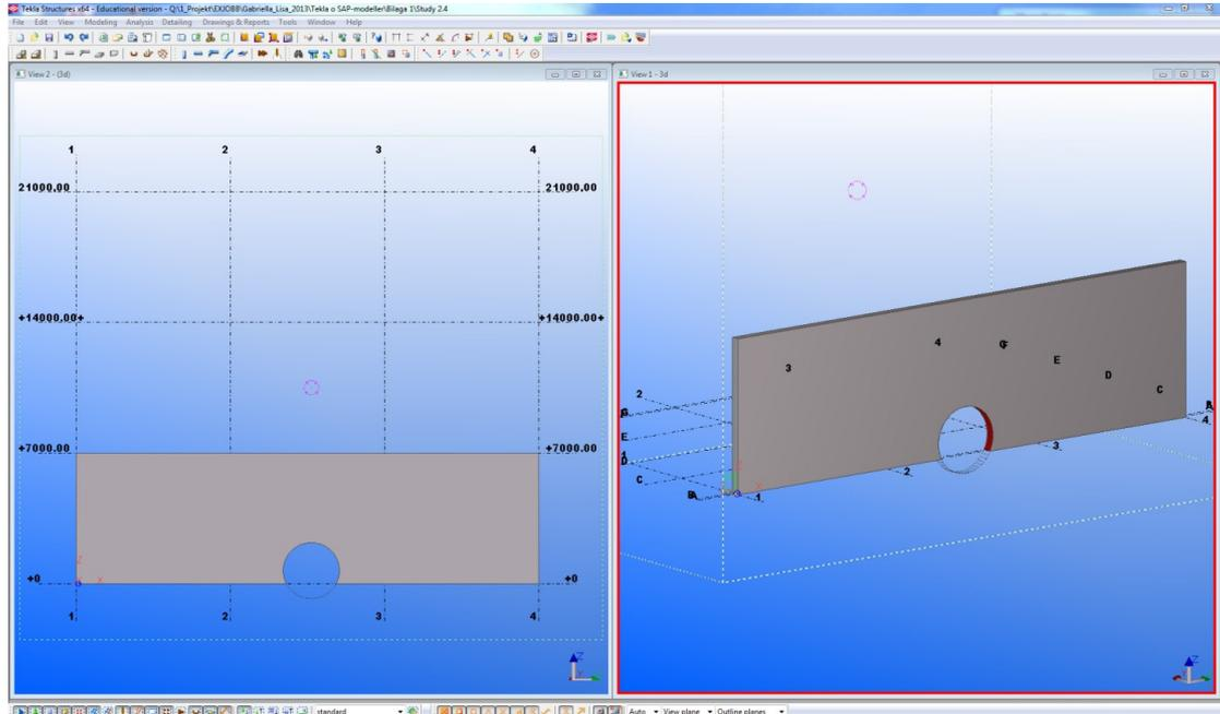
2. The *Analysis & Design model* was created. Analysis lines and nodes were generated for both the panel and the circular opening.
