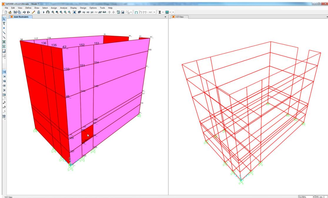
8. By opening the *Assign Automatic Area Mesh* box it could be seen that the program recommend the meshing option *No Auto Mesh*. The meshing option was changed to *Area Into Objects of This Maximum Size (Quads and Triangles Only)*. The maximum size chosen by the program was kept.
