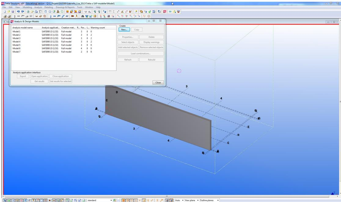
3. An *analysis & design model* was created. Analysis lines were displayed as highlighted yellow lines with nodes at the corners. During the creation of the *analysis & design model*, warning counts can appear. These must always be controlled by the user, and if necessary be fixed.
