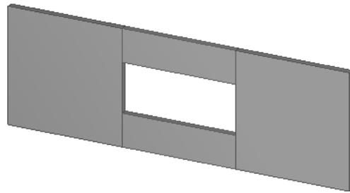
*Figure 3.14 Several panels modelled to create an opening in the model.*
