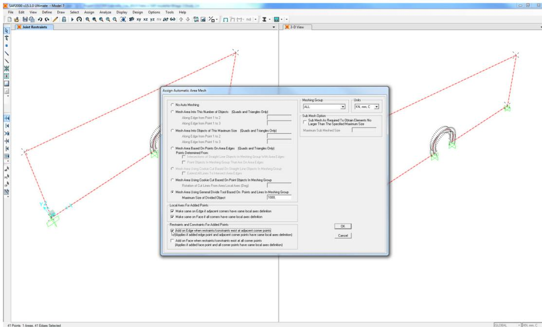
7. An analysis was performed but it was stopped by an error message. This may be caused by the too closely spaced nodes in the opening.
