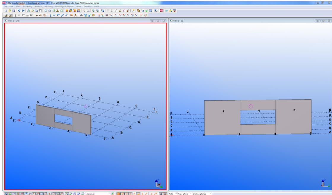
2. An *Analysis & Design model* was created. Analysis lines were created for each panel-part and the elements shared an analysis line.
