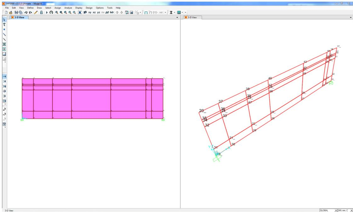
13. The number of the nodes of the opening was localised by comparing with numbers in the analysis model in TS. The area in between the nodes for each opening was selecting by marking the area and pressing *delete*.
