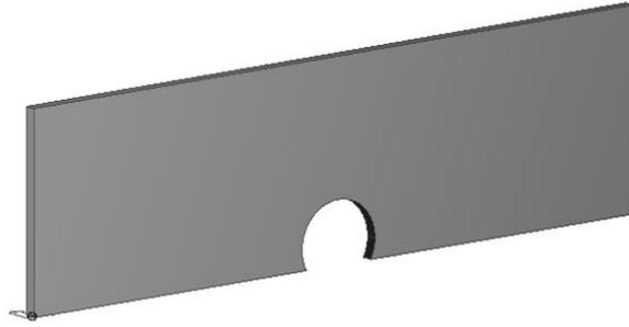
*Figure 3.29 Circular opening modelled at the edge of a panel.*
