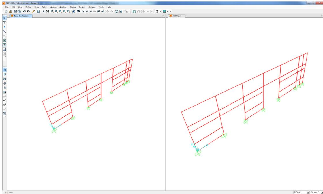
11. By opening the *Assign Automatic Area Mesh* box it could be seen that the program recommend the meshing option *No Auto Mesh*. The meshing option was changed to *Area Into Objects of This Maximum Size (Quads and Triangles Only)*. The maximum size chosen by the program was kept.
