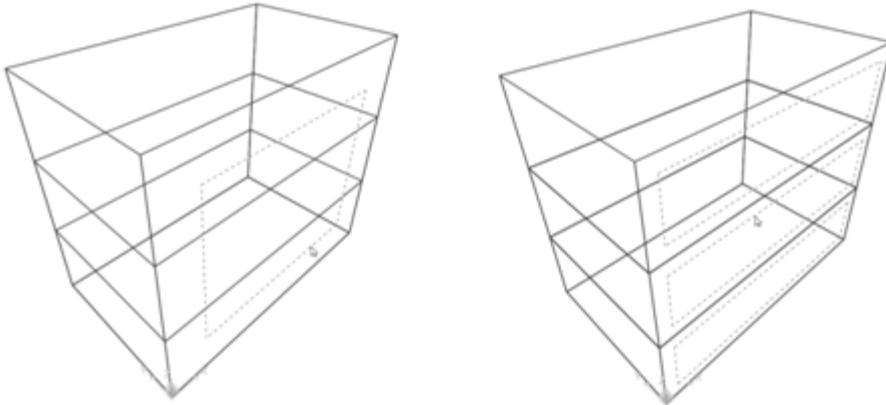
*Figure 3.9 To the right: a model with three panels upon each other, one top panel is highlighted, exported to SAP. To the left: A model with one panel spanned all the way from the bottom to the top. The entire panel is highlighted, exported to SAP.*
