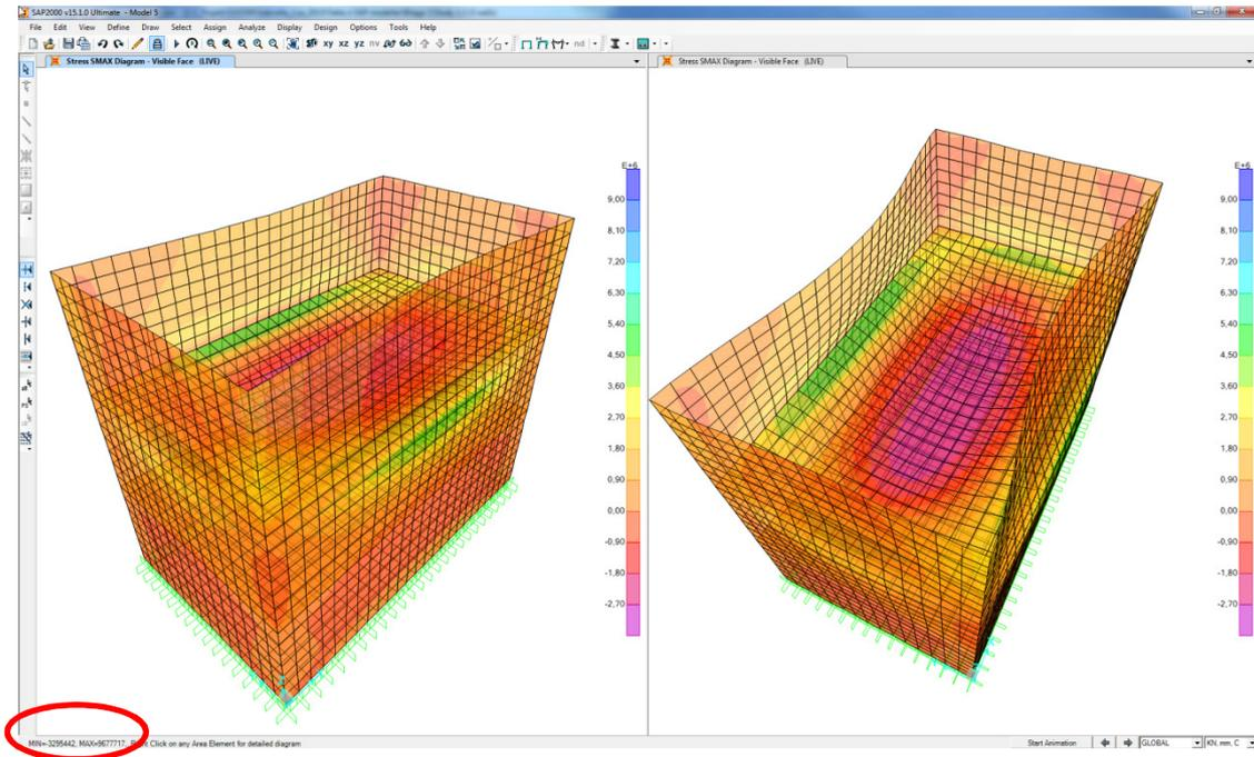
10. For the second case, the model was created with one panel element along all three floors otherwise the same modelling technique was used as for the previous model.
