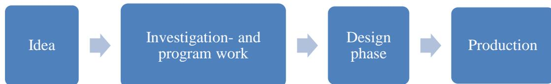
Figure 2.1 Stages in a building project
