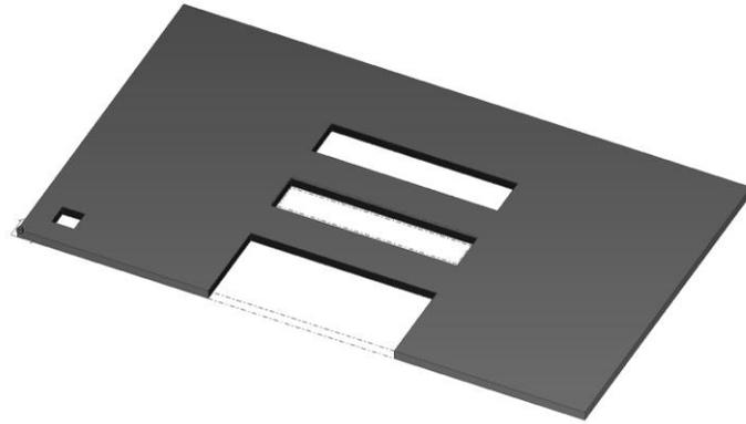
Figure 3.32 Openings within and at the edge of a slab modelled in TS.
