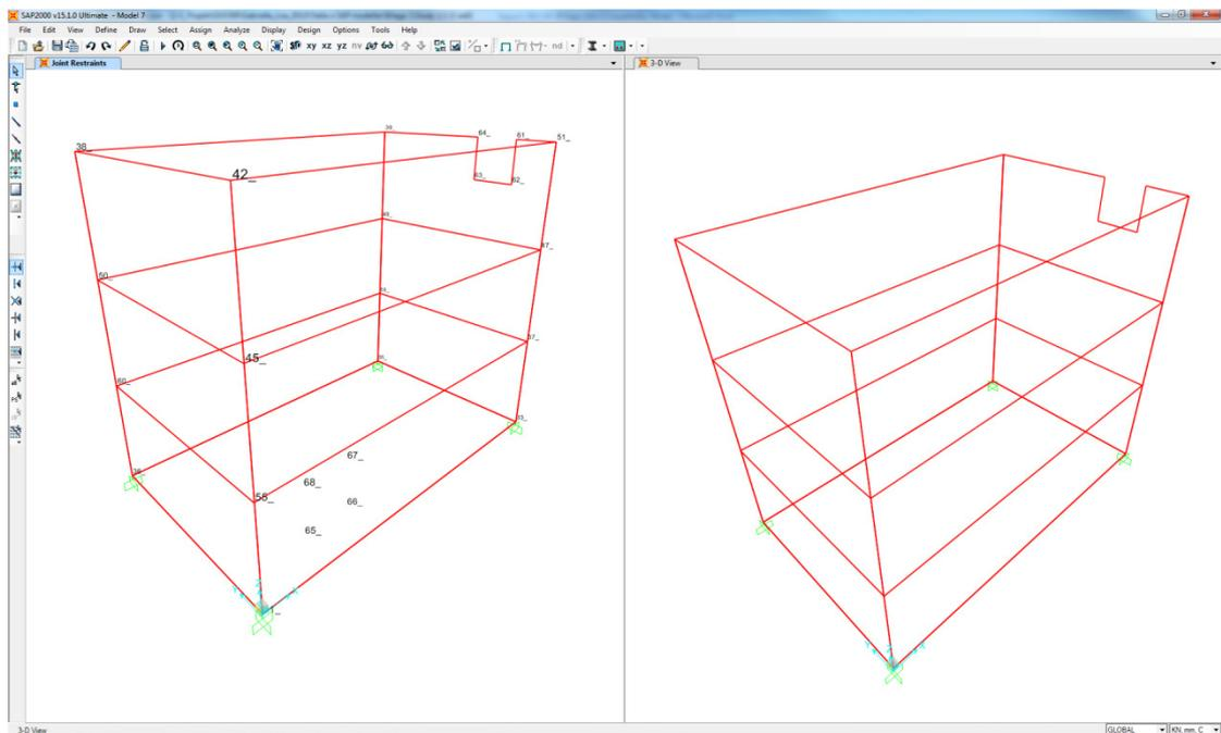
5. The model was divided into smaller areas in the *Divide Selected Area* box by choosing the option *Divide Area Using Cookie Cut Based On Selected Point Objects with the Rotation of Cut Lines From Area Local Axes*.
