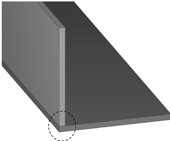
*Figure 3.5 Connected surfaces of the concrete slab and the concrete panel.*
