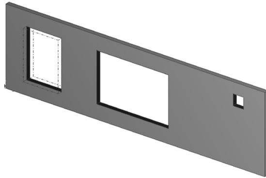
*Figure 3.10 Openings modelled within a panel in TS using different modelling techniques.*
