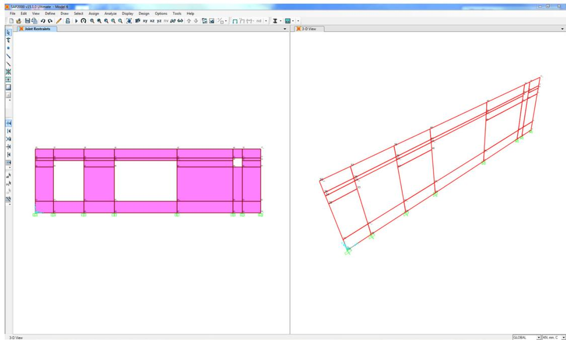
15. By opening the *Assign Automatic Area Mesh* box it could be seen that the program recommend the meshing option *No Auto Mesh*. The meshing option was changed to *Area Into Objects of This Maximum Size (Quads and Triangles Only)*. The maximum size chosen by the program was kept. In order to get a sufficient fine mesh the option *Sub Mesh As Required To Obtain Elements No Larger Than The Specified Maximum Size* was used and a maximum size of the elements was specified.
