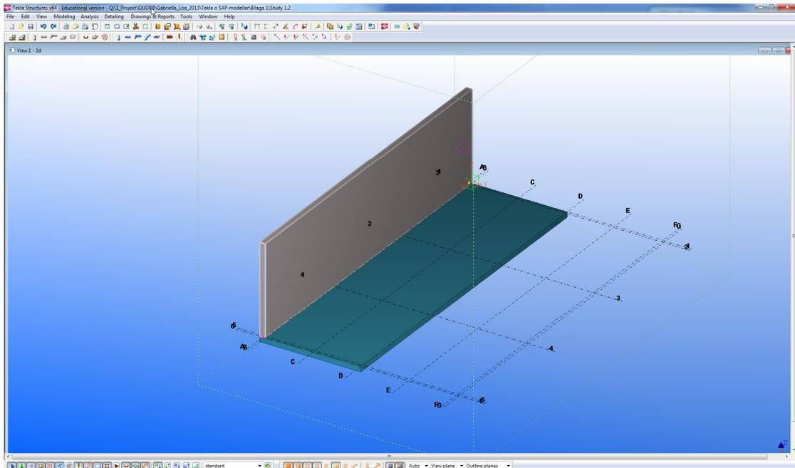
2. The panel was modelled in connection to the surface of the slab.
