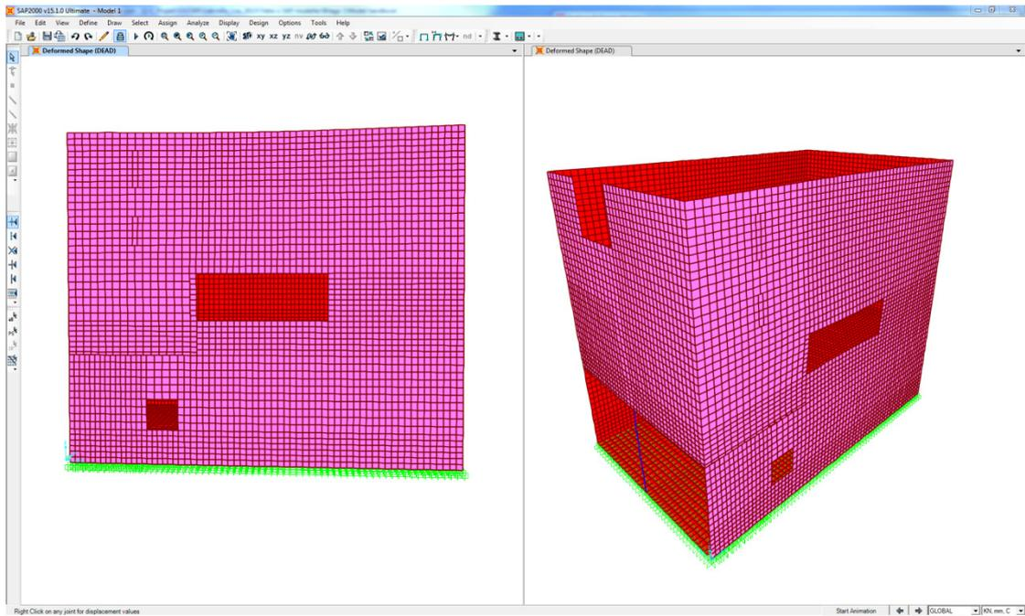
The model is analysed influenced only by dead weight and the result is displayed by a deformed shape. The new mesh which is generated is finer.
