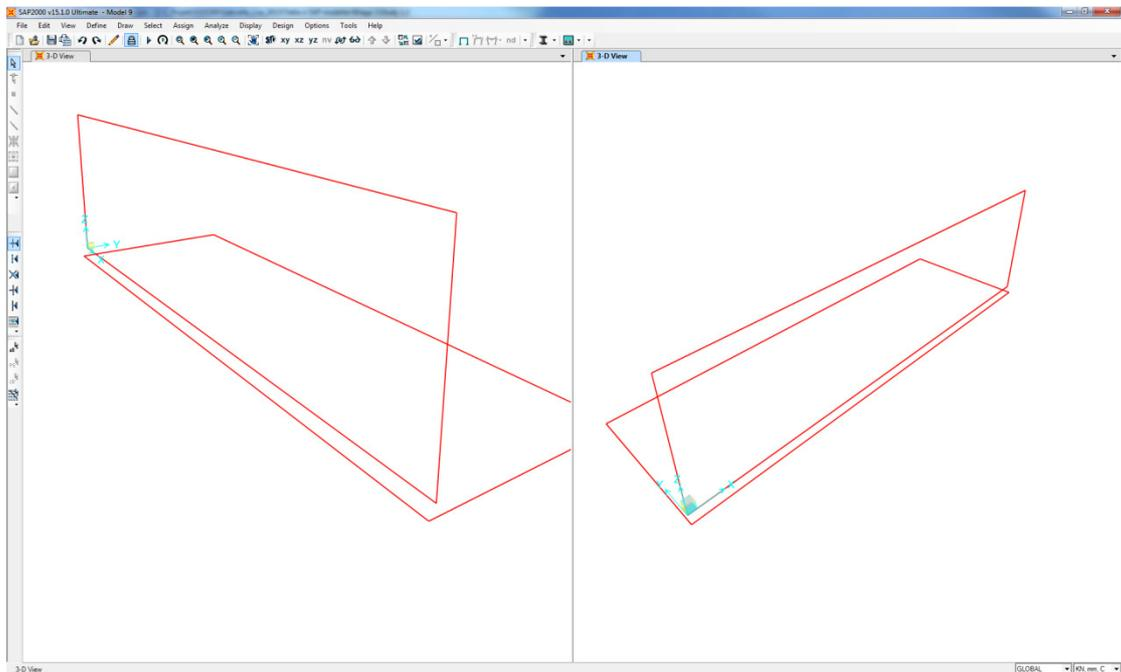
5. The modelling was redone and instead the panel and the slab were connected to each other in their centre lines.
