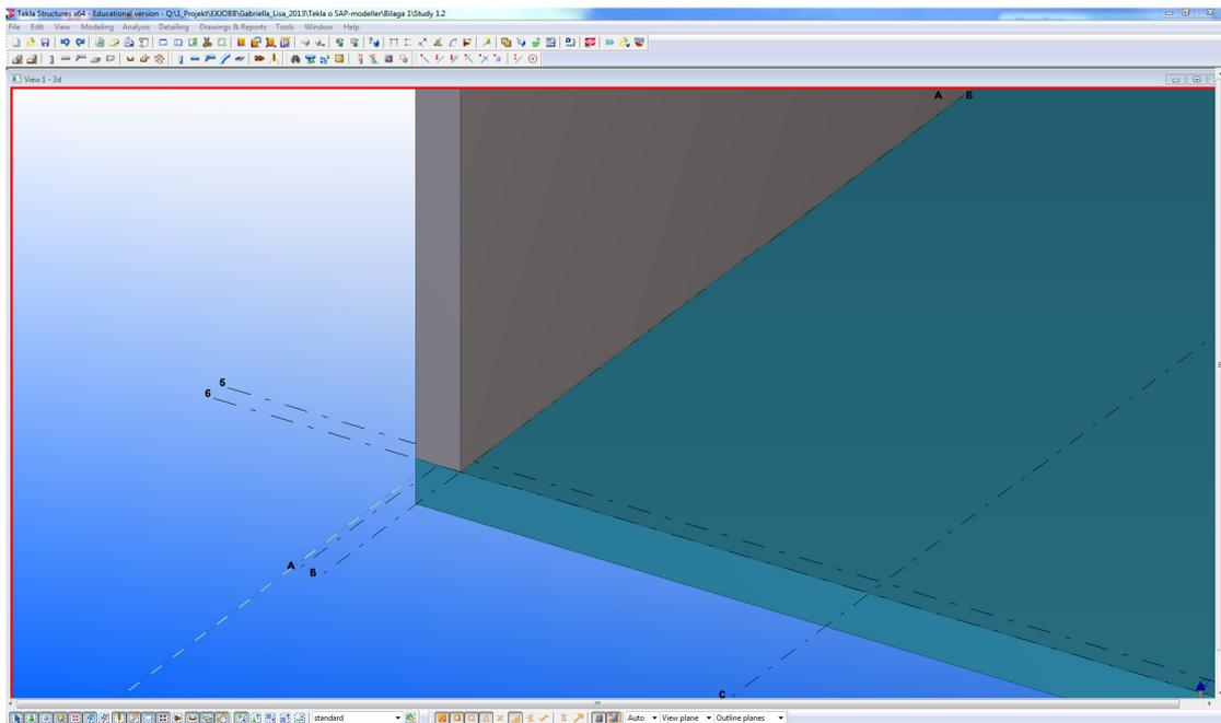
3. The *Analysis & Design model* was created and two separated analysis lines were obtained in TS.
