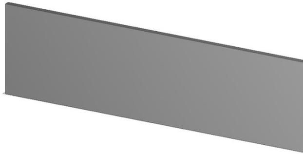
*Figure 3.4 A model of a single concrete panel modelled in TS and exported to SAP.*
