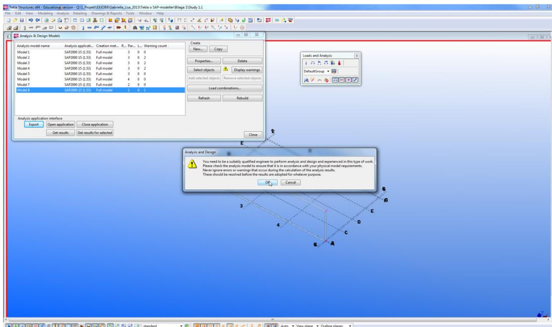
8. The model was exported to SAP by clicking on the *Export*-bottom and SAP was automatically started. Note: SAP opens with the units kN, mm and C.
