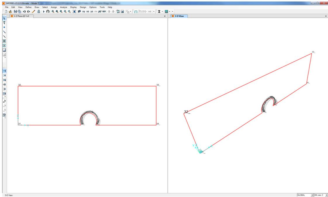
4. The nodes along the bottom edge of the panel were fully restrained.
