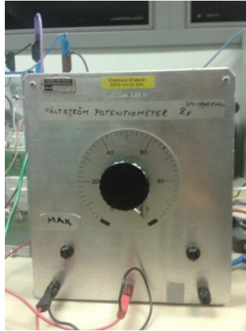
Figure 4.9: Potentiometer used in the battery role.
