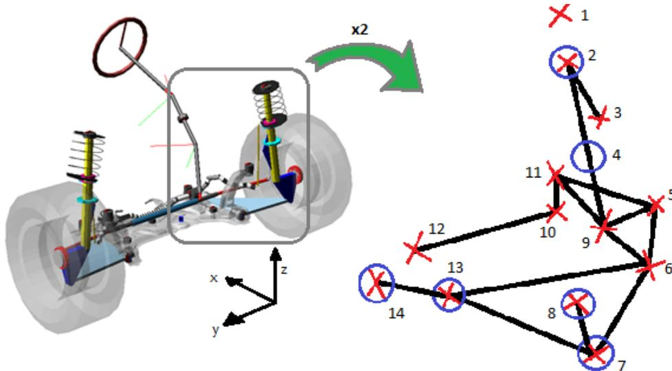
Figure 4: McPherson strut front suspension assembly and structural model
