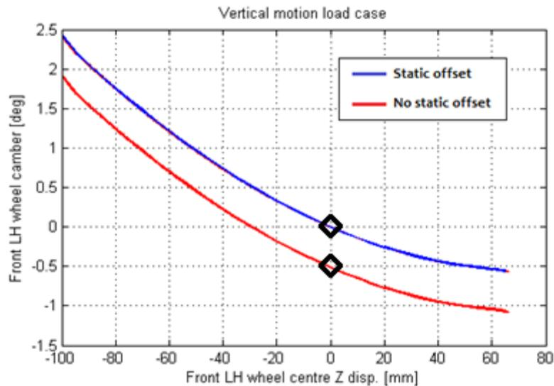
Figure 11: Static offset of suspension characteristics
