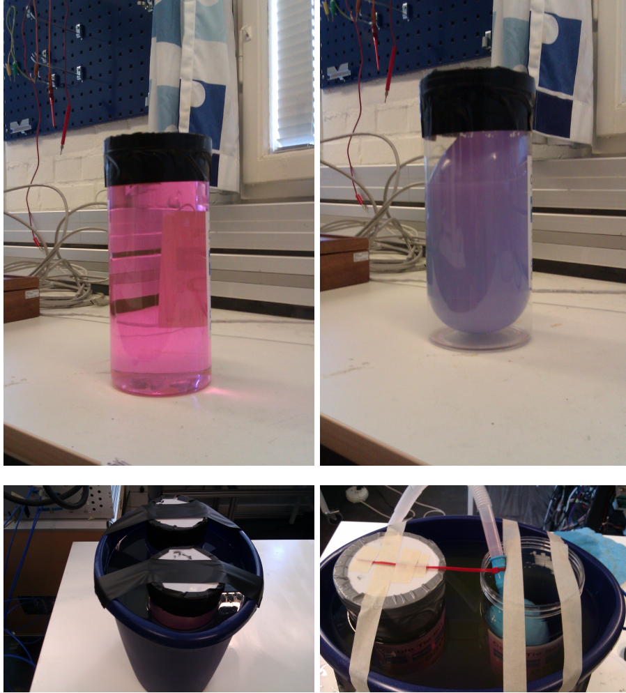
Figure 2.3: Pictures of: (a) A cylinder modelling a healthy lung (b) A cylinder modelling a 20% PTX (c) Assembled thorax phantom (d) Setup for continuous measurements of a decreasing PTX.
