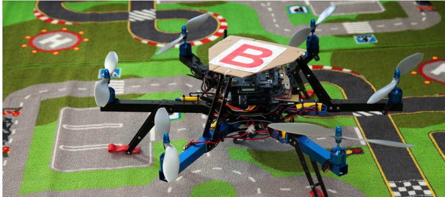
Figure 37: Hexacopter ready for system evaluation with letter B mounted on its back to enable tracking using ceiling camera.
